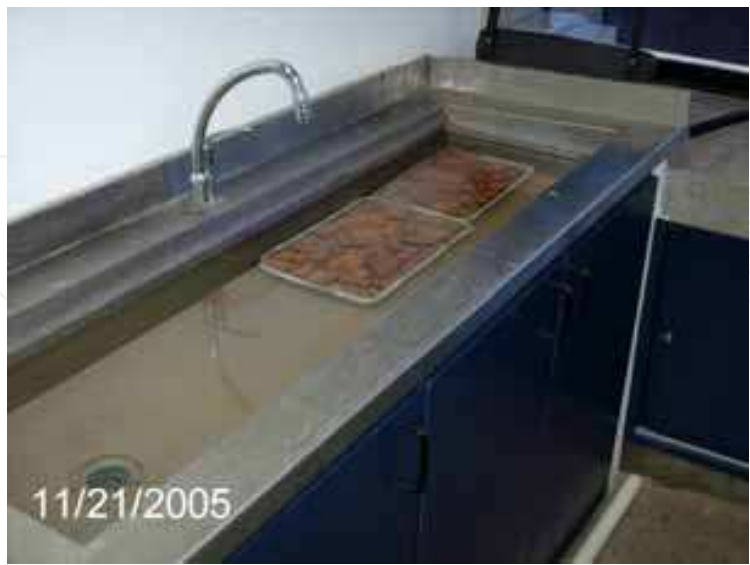
Fig. 10. Laboratory tank for wetting and drying cycling test
