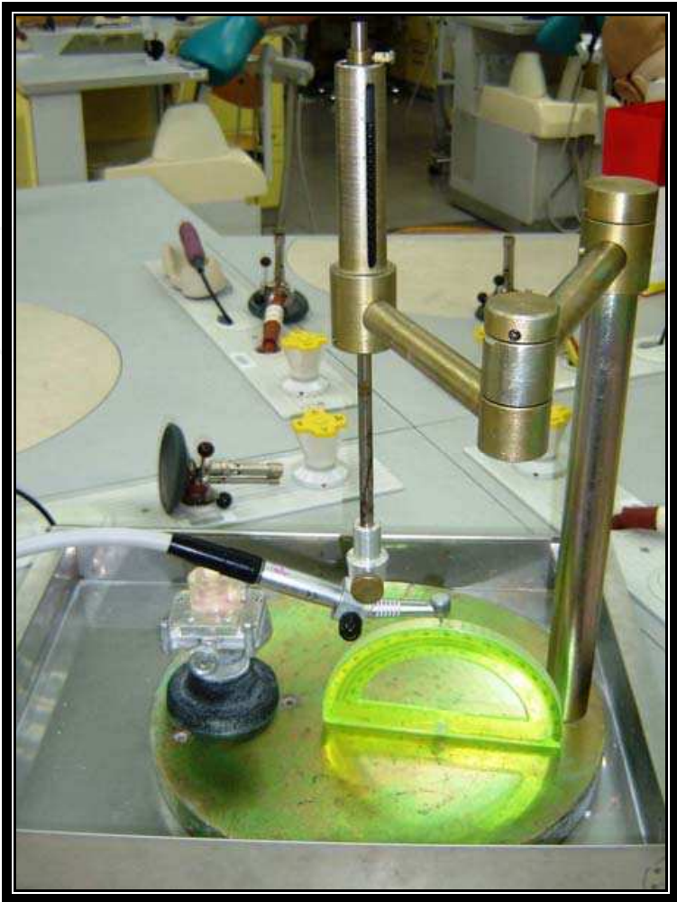
Fig. 2. The paralleling apparatus used
