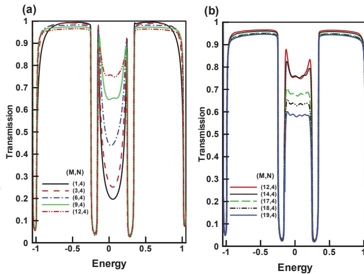
Fig. 5. Transmission through graphene ribbon with 4 zigzag chains in width for different ribbon lengths: a)  $M \leq 12$  b)  $M \geq 12$ . Applied bias is considered to be  $0.5V$ . Edge impurity changes onsite energy of the edge atoms as  $\varepsilon_\alpha = 0.1t$ .
