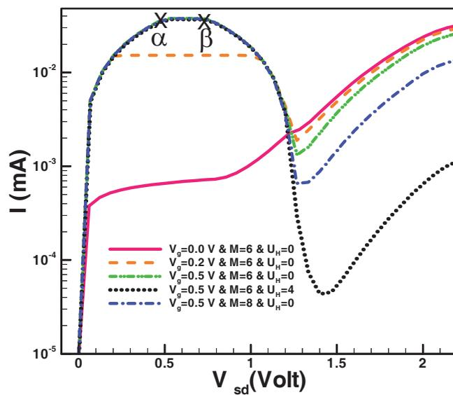
Fig. 6. Current-voltage characteristic curve for different gate voltages when the ribbon size is as  $(N, M) = (4, 6)$ . The effect of different parameters such as size effect, electrostatic potential and also gate voltage is investigated on I-V curve. Hubbard parameter ( $U_H$ ) is on site Coulomb repulsive.
