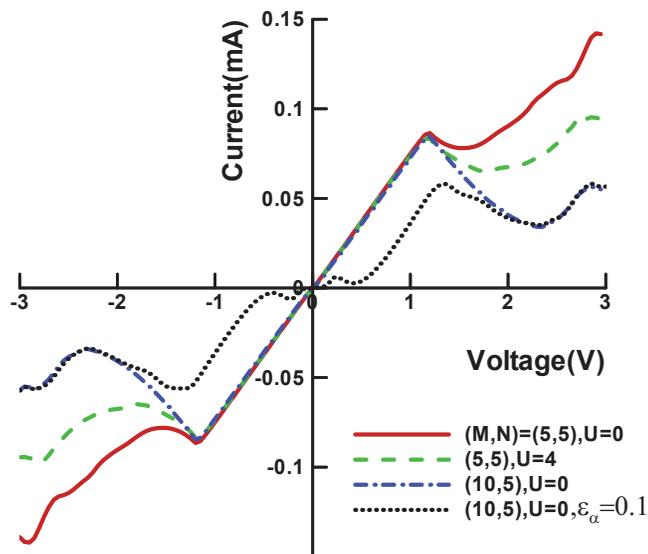
Fig. 10. Current-voltage characteristic curve of an odd zigzag graphene nanoribbon with  $N = 5$  (zigzag chains). I-V curves are compared for two ribbon lengths;  $M = 5$  and 10. For the case of  $(M, N) = (5, 5)$  and for comparison purpose, I-V curve is also plotted in the presence of electron-electron interaction ( $U$ ). NDR phenomena is preserved when one of the ribbon edges is doped by slight impurity (as  $\varepsilon_\alpha$ ).
