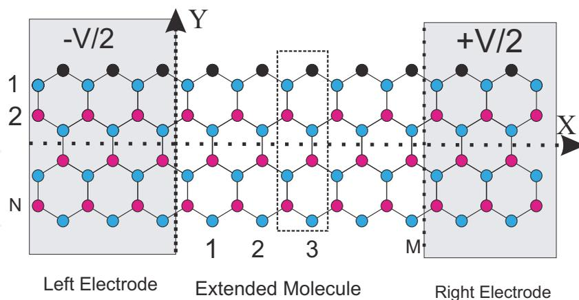
Fig. 3. Even asymmetric zigzag graphene nanoribbon considered as a central region attached to two electrodes. Transverse zigzag carbon chains and unit cells inside the central region are labeled by N and M. Darker edge atoms are absorbed atoms which make ribbon asymmetric in respect to the X-axis.
