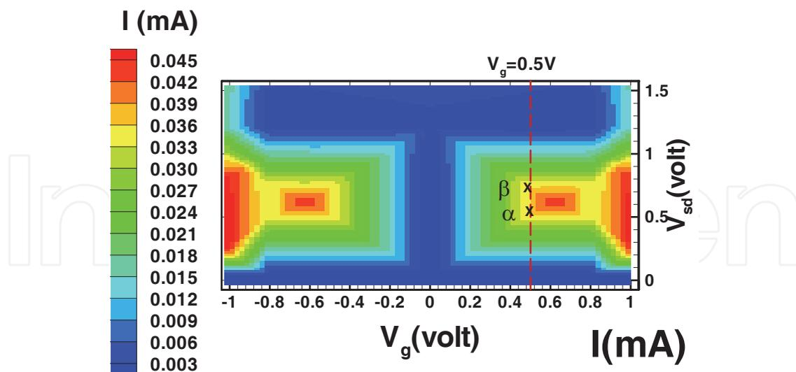
Fig. 8. Contour plot of the current in terms of  $V_{sd}$  and  $V_g$  for a zigzag graphene nanoribbon with  $(N,M)=(4,6)$ . Vertical dotted line corresponds to  $V_g = 0.5V$ .  $\alpha$  and  $\beta$  are those points which was shown in Figs(6,7).
