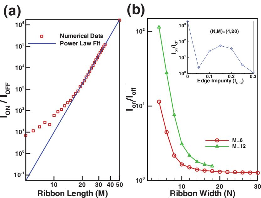
Fig. 9. a) On-off ratio of the current increases as a power law with the ribbon length for  $N = 4$  and  $V_g = 0.5V$ . b) On-off ratio of the current decreases with the ribbon width (circle and triangular points) while it is disappeared for edge impurity (diamond points) stronger than  $0.3t_{C-C}$  (inset figure).
