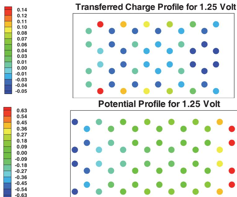
Fig. 14. Transferred charge and Electrostatic potential profiles for  $V_{sd} = 1.25$  volt and  $V_g = 0.5$  volt in the weak screening case. Due to charge transfer through the ribbon edges, screening is so weak that the external potential can penetrate inside the central portion.
