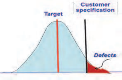
Fig. 3. Concept of Variation and Defects
