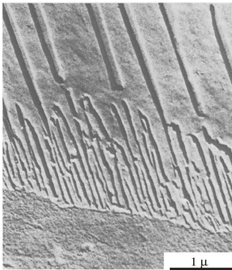
Fig. 17. Secondary electron micrograph of low-alloy steel partially transformed to pearlite at 700°C for 15 minutes and then quenched. Finer-scaled pearlite near the transformation front was probably created by a rapid growth during the quenching. Note oblique angle of the pearlite structure to the transformation front. From Darken and Fisher (1962) Figure 2, used with permission
