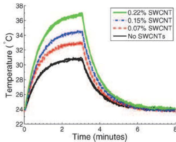
Fig. 15. Microwave heating response of tissue mimic materials with various concentrations of carbon nanotubes. Each curve shows the temperature profile of a sample that was heated via 3-GHz microwave illumination for 3 min and allowed to cool for 5 min. (Mashal *et al.* 2010)
