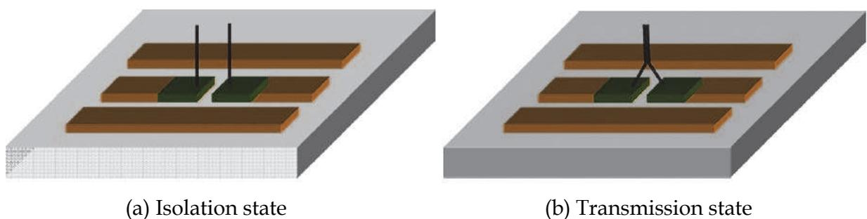
Fig. 10. Architecture of Carbon nanotube ohmic switch (Demoustier 2008)
