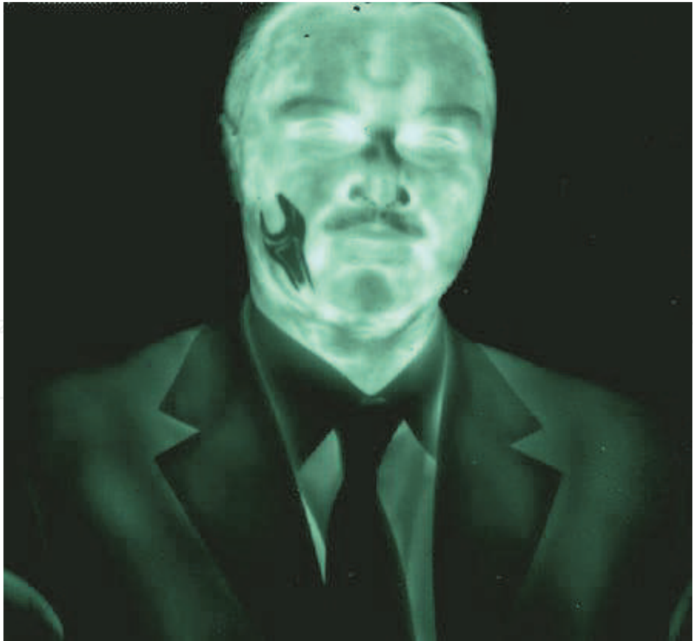
Fig. 19. Thermal image obtained from 640×512 array based on HgCdTe/CdTe/ZnTe/Si(310)
