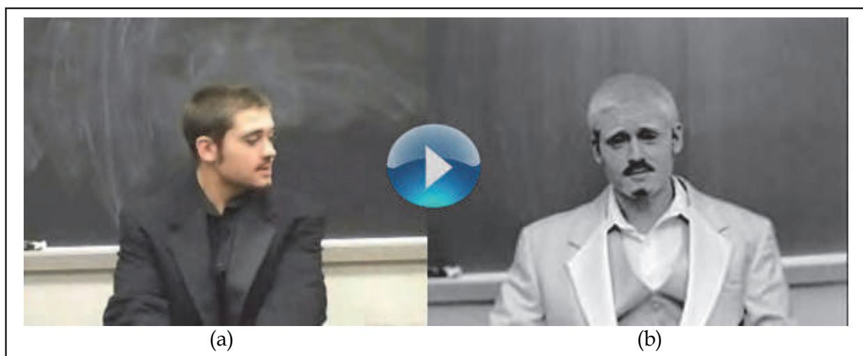
Fig. 5. (a) an actor wearing typical stage make up in color image, (b) same actor in SWIR band ( http://sensorsinc.com/border_security1 ).
