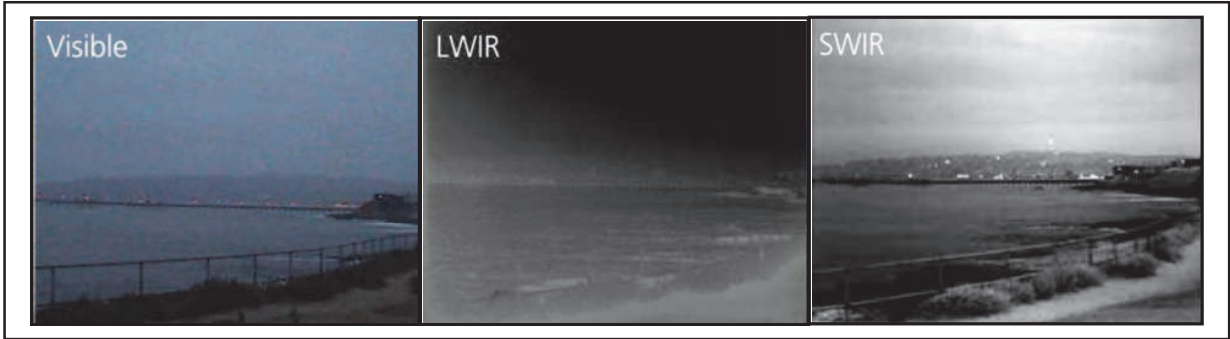
Fig. 3. At sunrise SWIR cameras provide effective imaging day and night thus eliminating thermal crossover.
