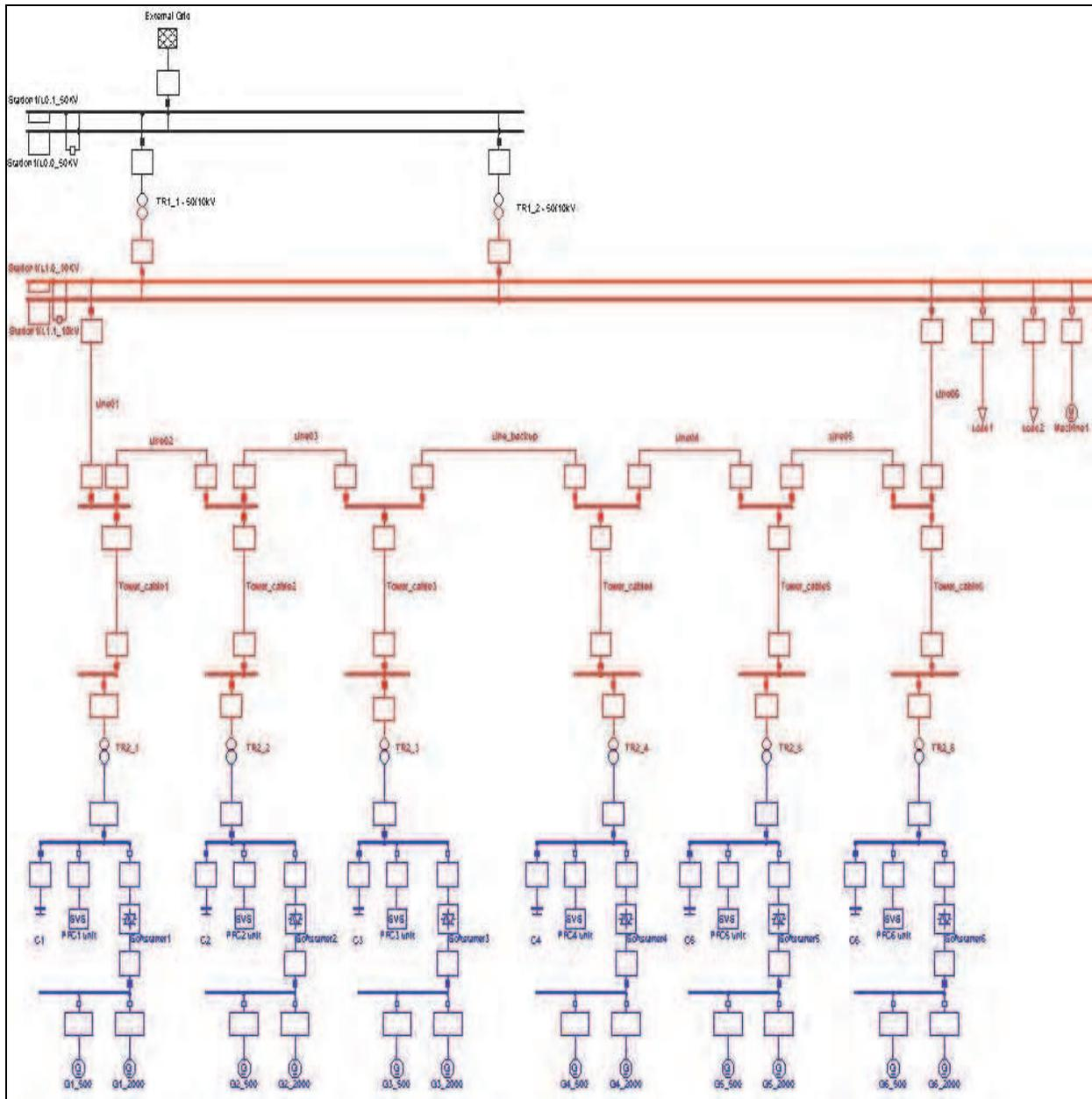
Fig. 14. 12 MW wind farm diagram implemented in Digsilent.
