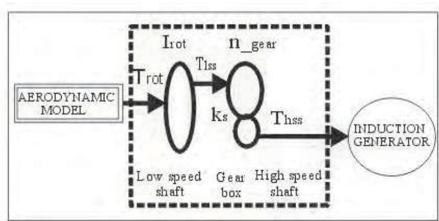
Fig. 4. Drive train model of the wind turbine.
