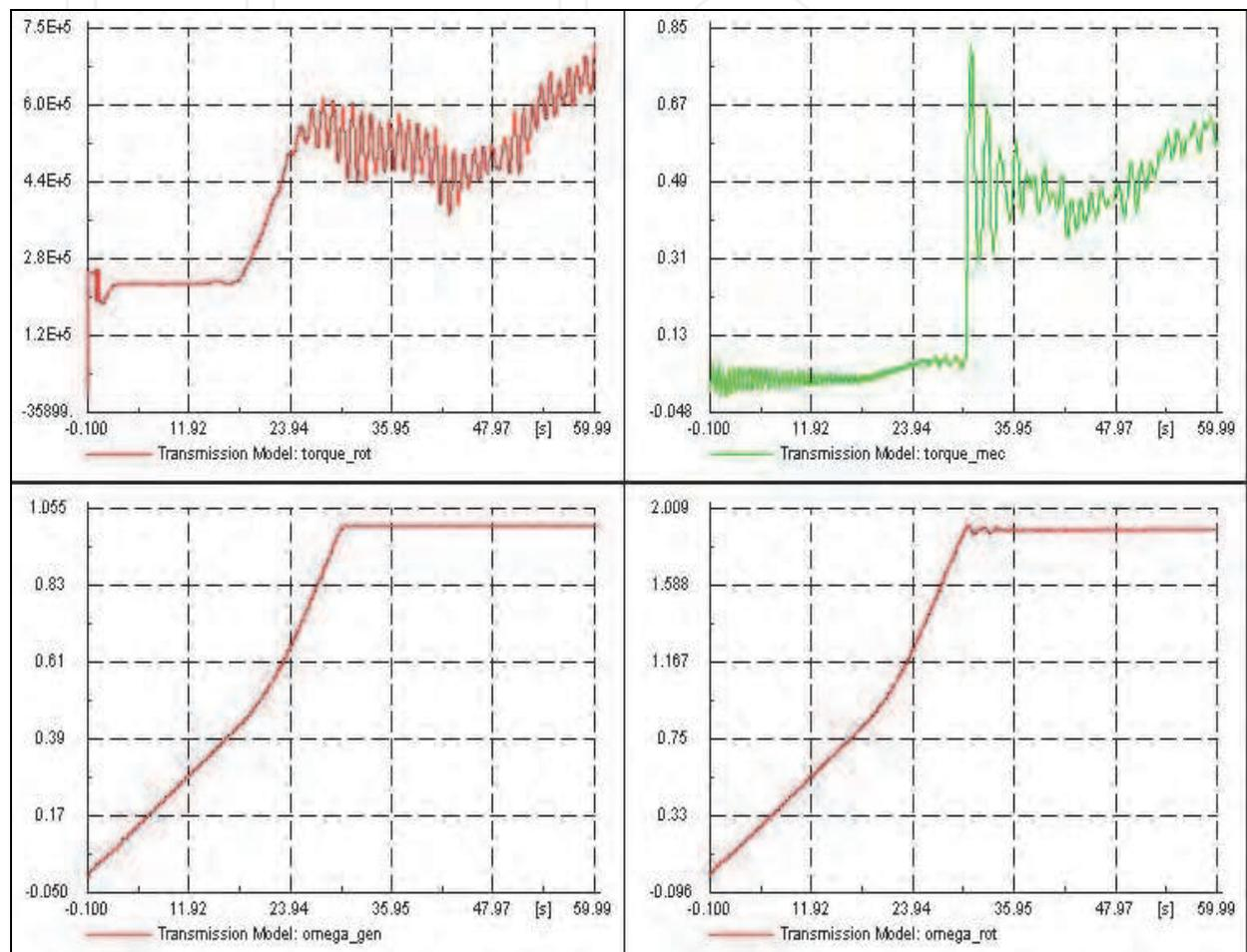
Fig. 16. Transmission model during start-up. Aerodynamic torque ( $\text{torque}_{\text{rot}}$ ), mechanical torque ( $\text{torque}_{\text{mec}}$ ), generator speed ( $\text{omega}_{\text{gen}}$ ) and rotor speed ( $\text{omega}_{\text{rot}}$ ) of wind turbine system.
