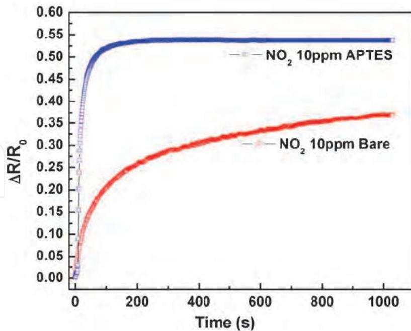
Fig. 17. Comparison of the normalized sensor responses to 10 ppm NO<sub>2</sub> gas between the SWCNT sensor on a bare and APTES-treated surface. Excepted from Tran et al.,2008. © Elsevier B.V.
