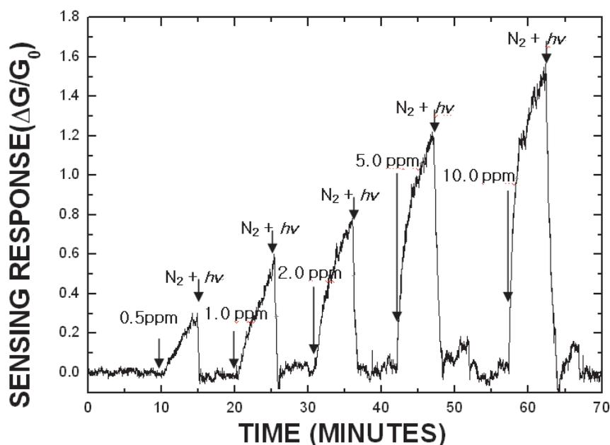
Fig. 19. The dependence of normalized sensing response of a SWCNT network sensor to the concentration of exposed  $\text{NO}_2$  gas at room temperature. Excepted from Maeng et al.,2008-a. © American Institute of Physics
