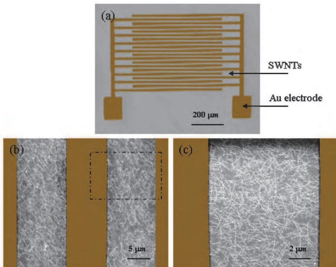
Fig. 15. (a) Optical image of the electrode arrays, where deposited SWCNT networks are separated by Au electrodes. (b) SEM image of SWCNT networks bridging Au electrodes deposited on Si/SiO<sub>2</sub> substrate. (c) An enlarged SEM image of (b). Excepted from Wang et al.,2006. © IOP Publishing Ltd
