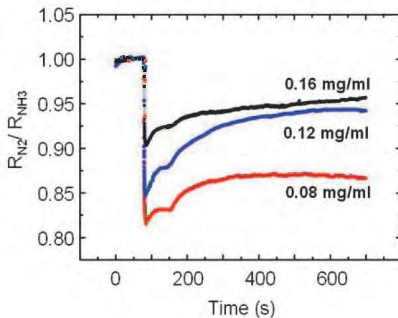
Fig. 10. Normalized sensor responses to the 50% NH<sub>3</sub> gas diluted in N<sub>2</sub> for various sensors with different nanotube densities. Excepted from Cho et al.,2006. © Materials Research Society
