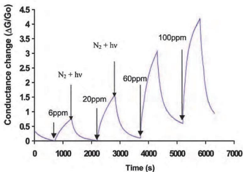
Fig. 7. Normalized sensor response of a drop-deposited SWCNT network sensor upon exposure to various concentration of NO<sub>2</sub> gas. Excepted from Li et al., 2003. © American Chemical Society
