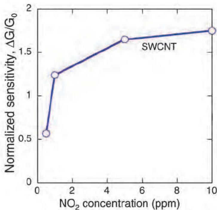
Fig. 14. The dependence of NO<sub>2</sub> gas concentration upon the normalized sensor response of a SWCNT network gas sensor fabricated by ac dielectrophoresis. Excepted from Suehiro et al.,2005. © Elsevier B.V.
