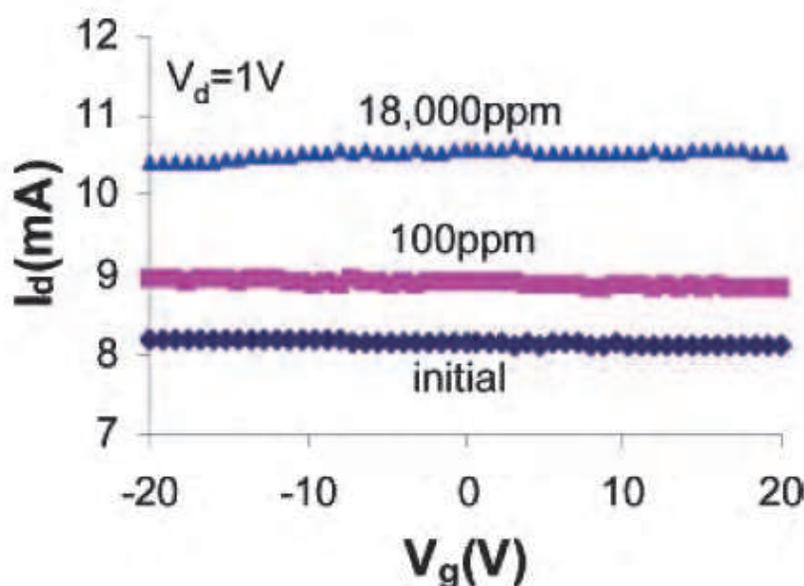
Fig. 12. Dependence of channel current upon gate bias of a SWCNT network FET fabricated by ac dielectrophoresis. The FET characteristics were measured at different  $\text{SOCl}_2$  concentrations. Small on/off ratio ( $\sim 1$ ) and vertical shift confirms that the charge transfer between SWCNT network and  $\text{SOCl}_2$  occurs mainly through metallic pathways. Excepted from Lee et al.,2006. © American Chemical Society
