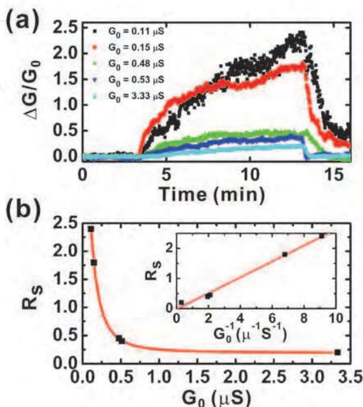
Fig. 20. (a) Normalized sensor response  $\Delta G/G_0$  of SWCNT network sensor to 500 ppb  $\text{NO}_2$  gas. (b) Sensitivity  $R_s$  vs base-line conductance  $G_0$  graph. (Inset) Sensitivity  $R_s$  linearly proportional to the inverse of the base-line conductance. Excepted from Maeng et al.,2008-a. © American Institute of Physics
