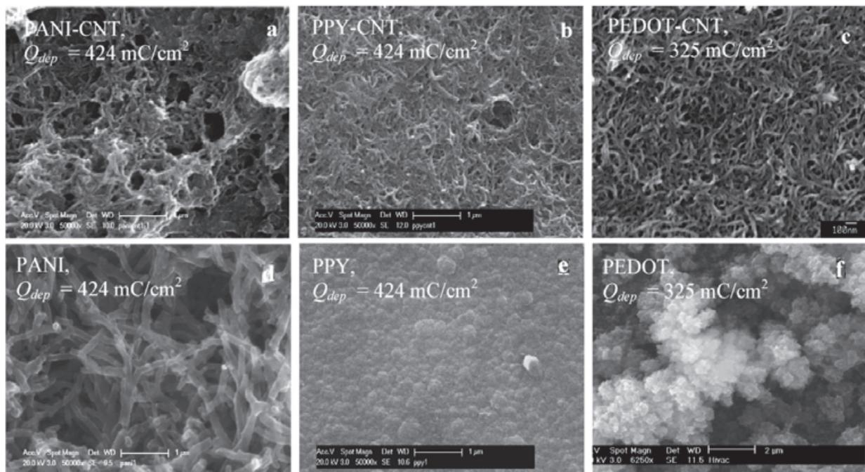
Fig. 3. SEM images of the surfaces of CNT composite films with polyaniline (PANI), polypyrrole (PPY) and poly[3,4-ethylenedioxythiophene] (PEDOT) (a–c) and of their pure polymer (d–f);  $Q_{dep}$  is deposition charges.
