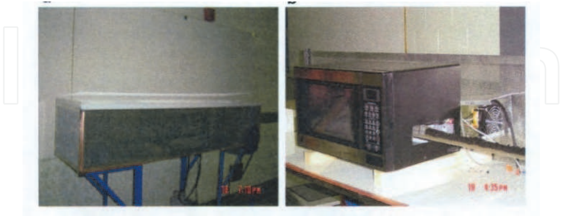
Fig. 5. (Left) Picture of the bench-scale microwave dewatering units with microwave shield in place. (Right) Close-up of the unit without the microwave shield showing the conveyor belt for feeding wet coal into the microwave oven (reproduced from the paper by Seehra et al., Fuel 2007).
