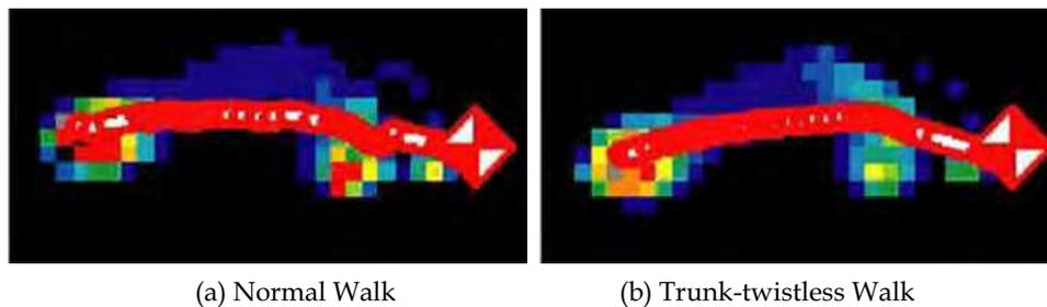
Figure 9. Trajectory of COP of Stance Foot
