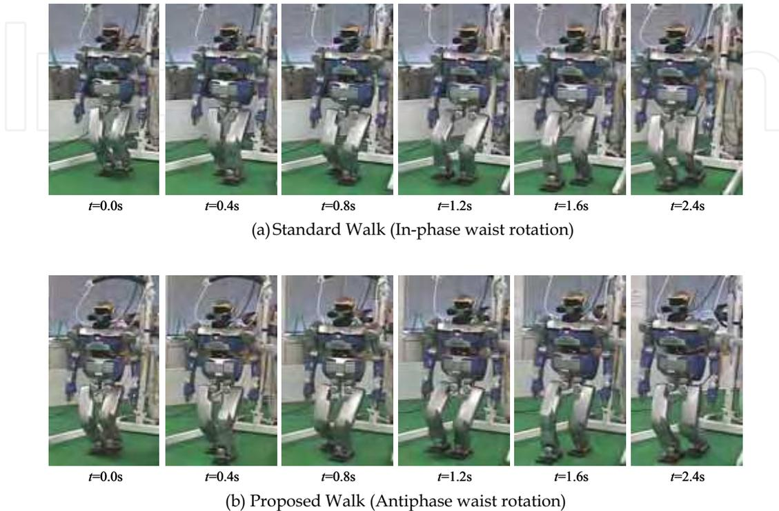
Figure 15. Experiments by Humanoid (0.83 km/h)
