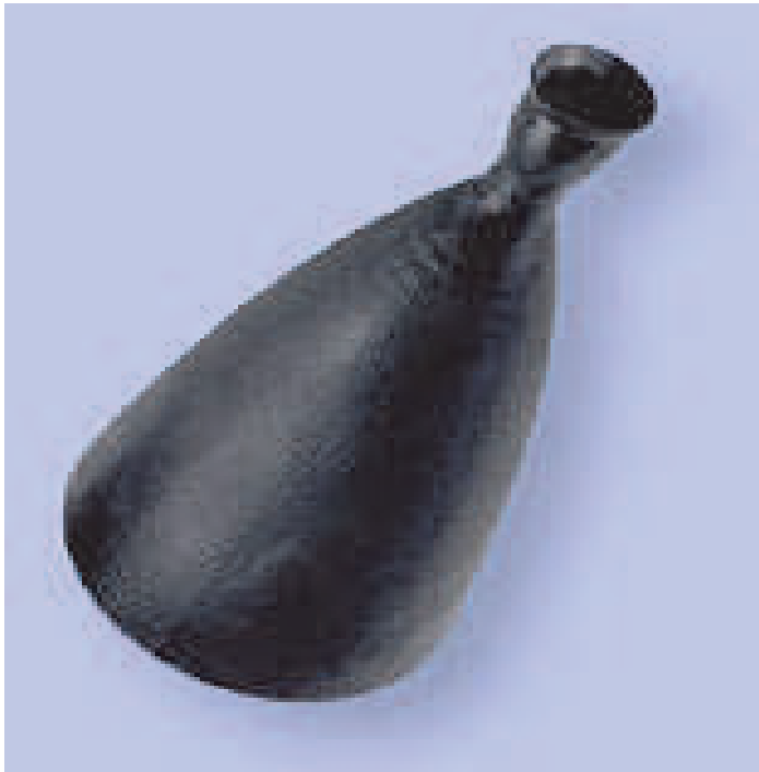
Fig. 4. Combustion chamber and nozzle of European Apogee Motor.
