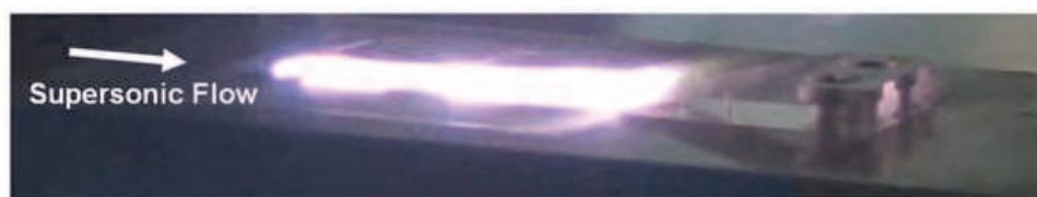
Fig. 3. Arc discharge picture in the supersonic flow.
