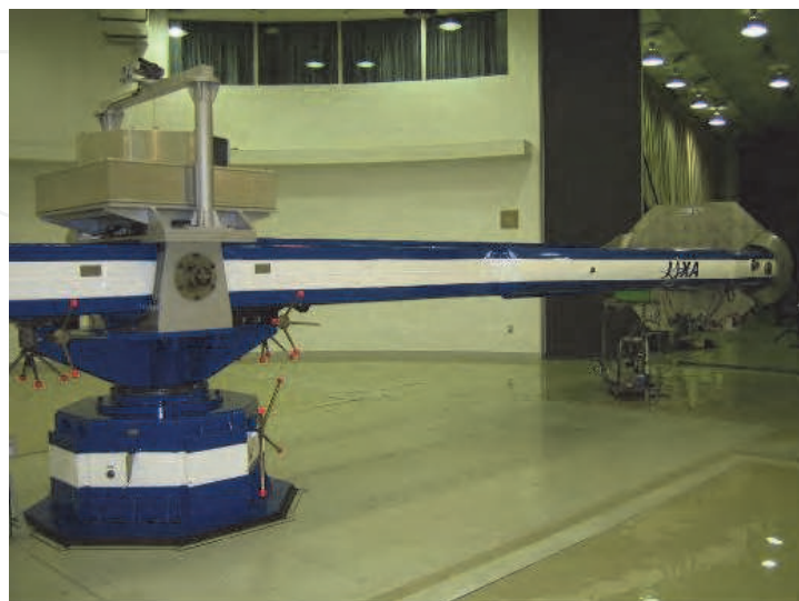
Fig. 12. Photograph of the rotation acceleration generator of JAXA.
