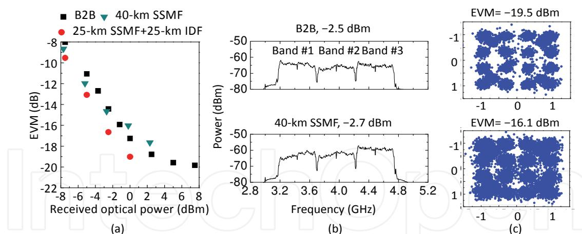
Fig. 9. Performance of the 60-GHz OFDM UWB signal measured at point (3) in Fig. 8 integrating optical and 5-m wireless transmission. (a) EVM for Band #1. (b) RMS spectrum (resolution bandwidth: 5 MHz). (c) Constellation diagrams for Band #1
