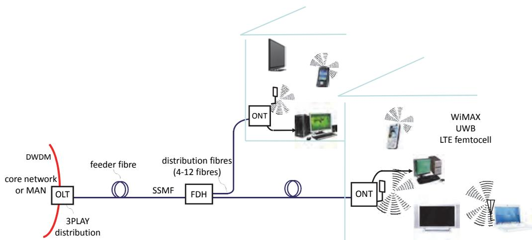
MAN: Metropolitan area network. OLT: Optical line terminal. ONT: Optical network terminal. SSMF: Standard single-mode fibre. FDH: Fibre distribution hub. DWDM: Dense wavelength division multiplexing
