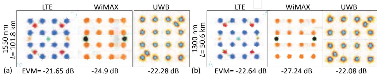
Fig. 5. Received constellations of LTE, WiMAX and UWB at different points of the experimental setup of Fig. 4: (a) after 101.8 km SSMF [Point (2)] for the 1550 nm downstream path, and (b) after 50.6 km SSMF for the 1300 nm upstream path
