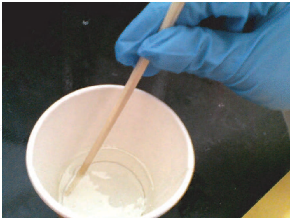
Fig. 3. Mixing of epoxy resin and hardener
