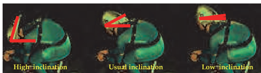
Fig. 11. Inclination of the head in time trial and corresponding inclination of the helmet (Wind tunnel of Marseille, France).
