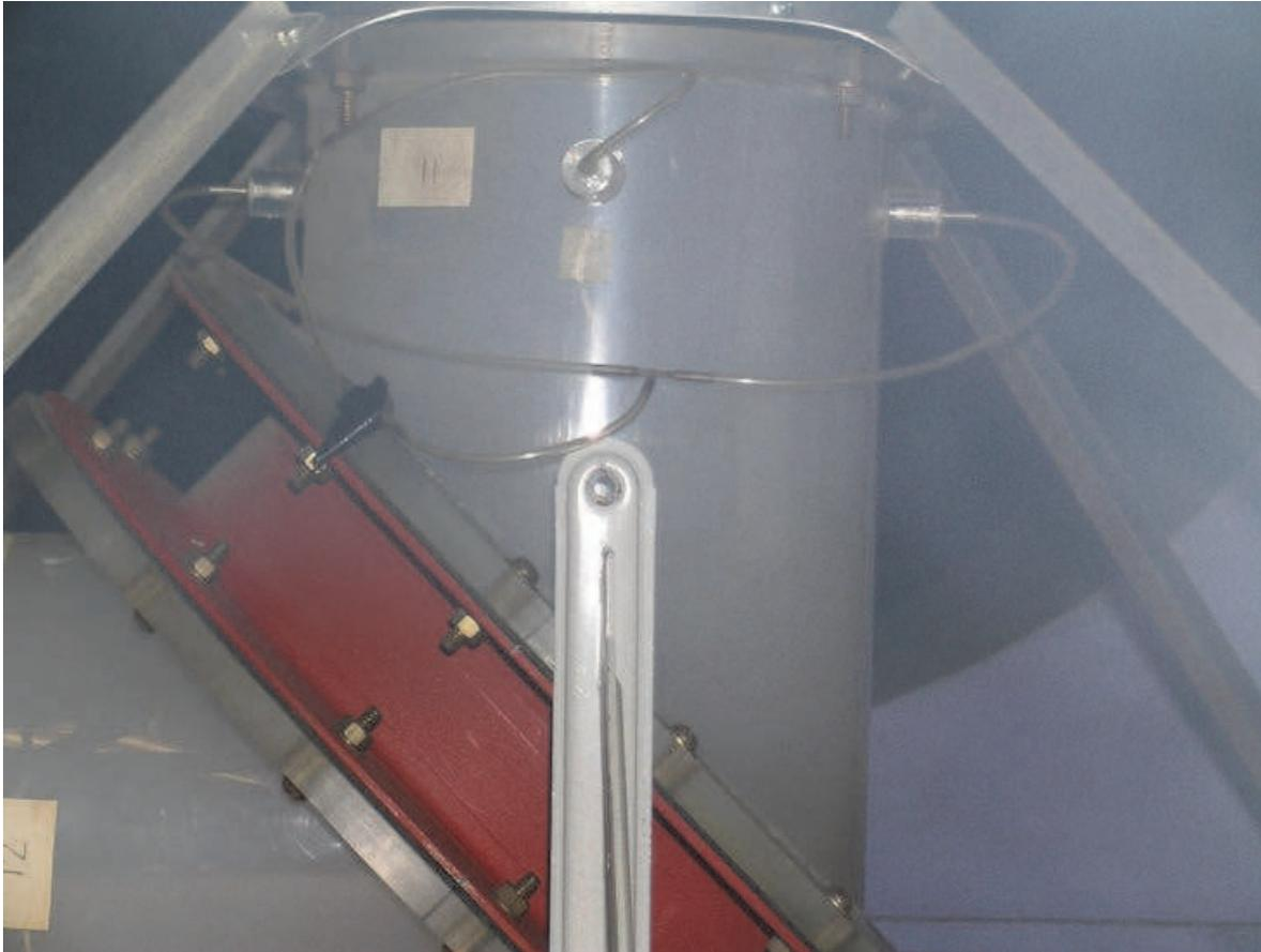
Fig. 22. Smoke flow visualisation at the intake.
