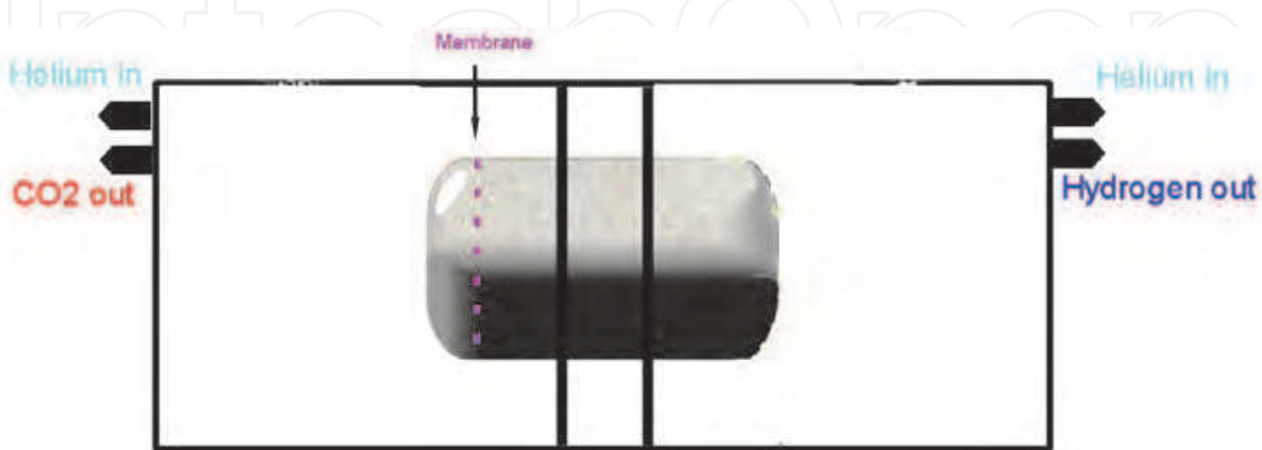
Fig. 3. Two dimensional conceptual model of the fuel cell without electrodes
