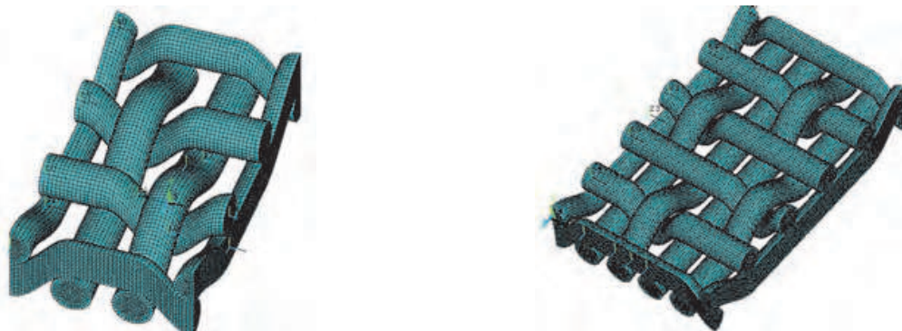
Fig. 11. Solid FE model of unit cell of twill (left) and satin (right) woven structure (Vassiliadis et al., 2008).
