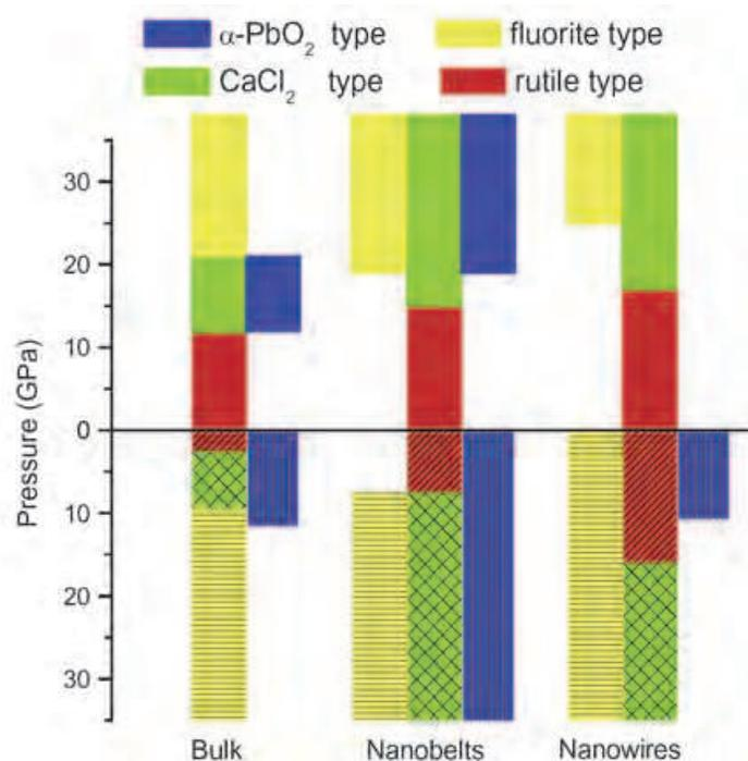
Fig. 10. Summary of pressure-induced phase transformations for SnO<sub>2</sub> nanobelts and nanowires upon compression (plain vertical bars) and decompression (hatched vertical bars) compared with those for bulk SnO<sub>2</sub> material. The different colors label different phases: rutile (red), CaCl<sub>2</sub> type (green), fluorite type (yellow) and  $\alpha$ -PbO<sub>2</sub> type (blue).
