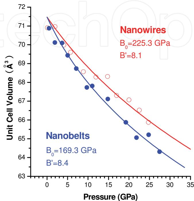
Fig. 9. Pressure-volume relations for SnO<sub>2</sub> nanowires (open circles) and nanobelts (solid circles). The solid lines are fittings using 3<sup>rd</sup> order Birch equation of state (see text).
