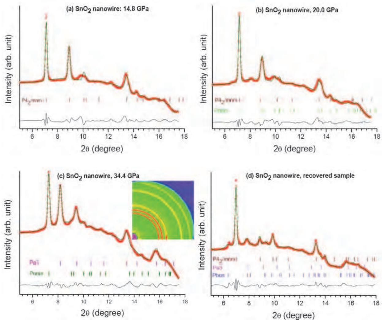
Fig. 8. Rietveld refinement of X-ray diffraction patterns of SnO<sub>2</sub> nanowires at 14.8 GPa (a), 20.0 GPa (b), 34.4 GPa (c) and from recovered sample (d). The legends follow Fig. 6.
