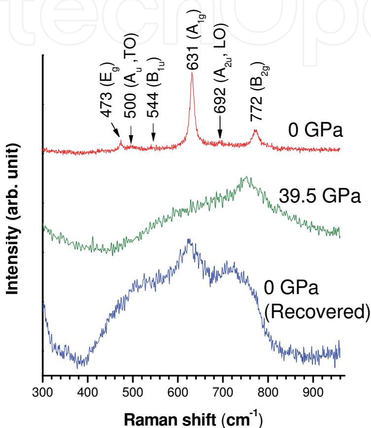
Fig. 4. Raman spectra of SnO<sub>2</sub> nanobelts in the spectral region of 300 to 1000 cm<sup>-1</sup> collected at ambient pressure (top), at 39.5 GPa (middle) and upon decompression (bottom). The assignments of the observed Raman modes are labeled above the ambient-pressure spectrum. (From Dong and Song, 2009)
