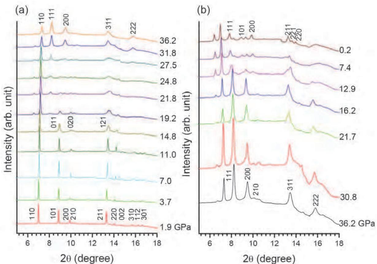
Fig. 5. X-ray diffraction patterns of SnO<sub>2</sub> nanobelts at selected pressures on compression (a) and decompression (b). Pressures in GPa are labeled along each pattern. The Miller indices are shown for the tetragonal structure at 1.9 GPa, the orthorhombic structure at 14.8 GPa and the cubic structure at 36.2 GPa on compression, and at 36.2 GPa and 0.2 GPa on decompression, respectively.
