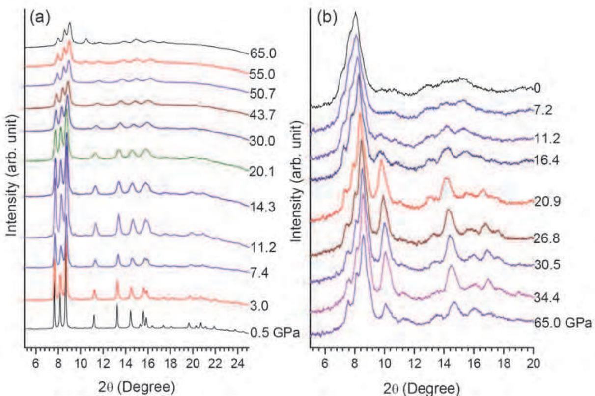
Fig. 11. Angle-dispersive X-ray diffraction patterns ( $\lambda=0.3680 \text{ \AA}$ ) of GaN nanowires at selected pressures upon compression (a) and decompression (b). The pressures in GPa are labelled along each pattern.
