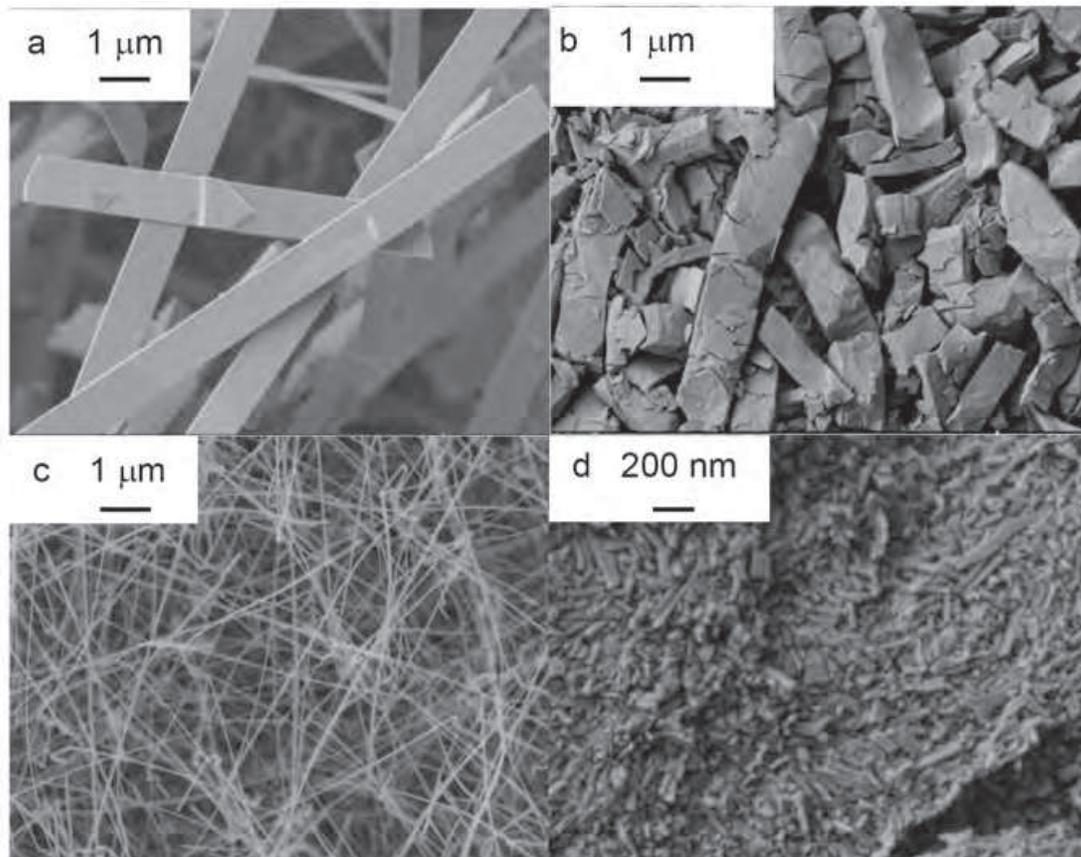
Fig. 1. SEM images of SnO<sub>2</sub> nanobelts before compression (a) and after decompression (b) as well as SnO<sub>2</sub> nanowires before compression (c) and after decompression (d) with scales shown in each panel. (From Dong & Song, 2009)
