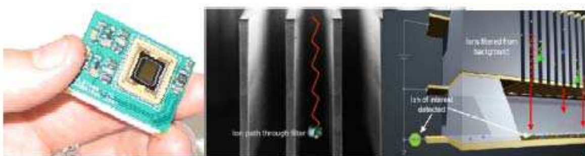
Fig. 4. FAIMS principle and chip of Owlstone Company
