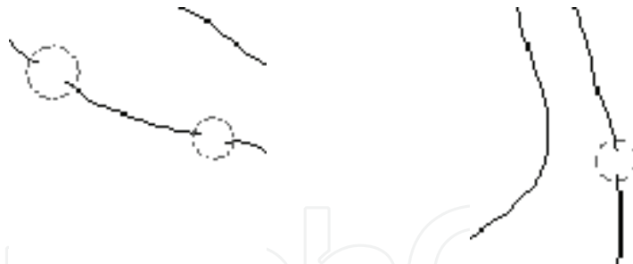
Fig. 10. Examples of union relationships. Some of the vessels present discontinuities leading to different segments. These discontinuities are detected in the union relationships detection process.
