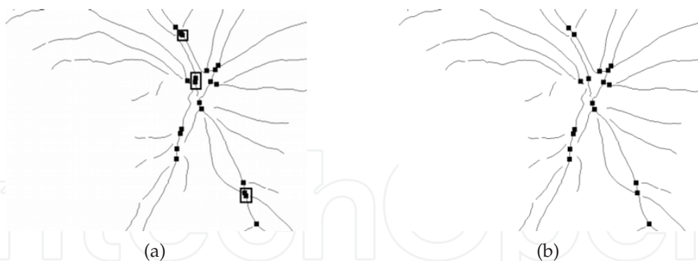
Fig. 15. Example of the result after the feature point filtering. (a) Image containing feature points before filtering. (b) Image containing feature points after filtering. Spurious points from duplicate crossover points have been eliminated.
