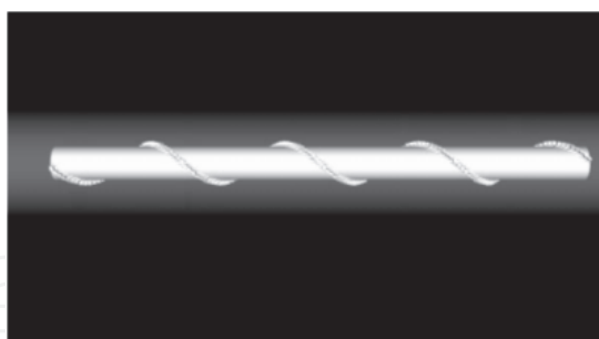
Fig. 1. Magnetic micro-machine (Adapted from Ishiyama et al., 2001)
