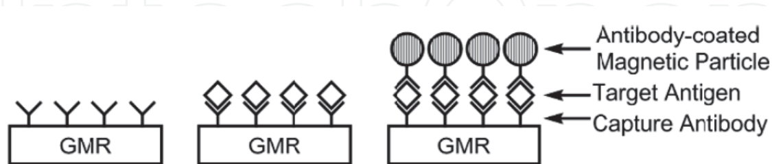
Fig. 13. Bacteria sensing using a GMR biosensor (Adapted from Millen et al., 2005).
