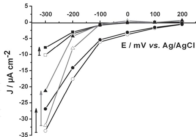
Fig. 17. Hydrodynamic voltammograms presenting the dependence of the sensor response for different electrode materials (gold - square, platinum - circles and graphite - triangles) modified with *H. polymorpha* "tr1" cells, recorded in the presence (filled symbols) and in the absence (opened-symbols) of L-lactate.
