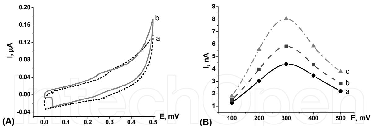
Fig. 1. (A) Cyclic voltammogram at a graphite electrode modified with adsorbed FC  $b_2$  (a) in the absence and (b) in the presence of 20 mM L-lactate (0 to +500 mV at a scan rate of 5 mV/s in 20 mM phosphate buffer, pH 7.2). (B) Hydrodynamic voltammograms obtained from a graphite electrode modified with adsorbed FC  $b_2$  in the presence of (a) 0.5 mM; (b) 1 mM; (c) 4 mM L-lactate in the absence of any electron-transfer mediator.
