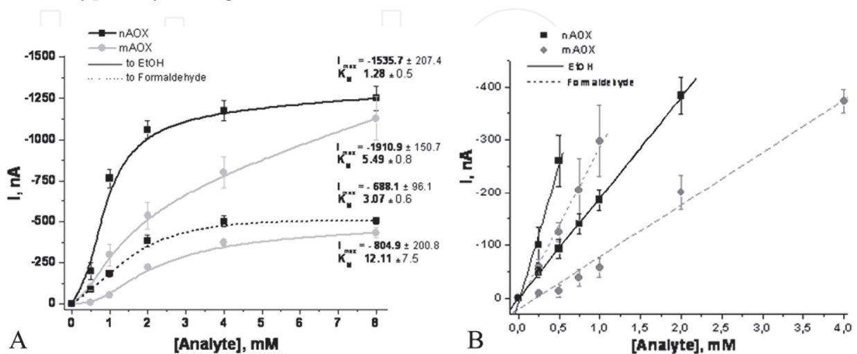
Fig. 26. Calibration curves and calculated  $K_M$  values of sensors based on the different forms of AOX toward ethanol (EtOH) and formaldehyde (A) and dynamic linear ranges of the corresponding sensors towards both analytes (B).
