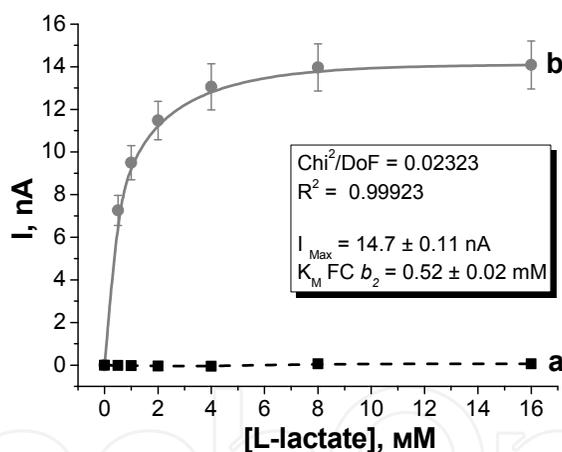
Fig. 2. Lactate calibration curve of a graphite electrode modified with adsorbed FC  $b_2$  at a potential of +300 mV and pH 7.2 in the absence of any redox mediator (b). Control experiment with a bare graphite electrode (a).
