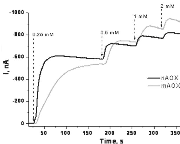
Fig. 25. Chronoamperometric assay of ethanol by *HRP/Os-Ap59//AOX/CP9* biosensors based on the natural (nAOX) and mutated (mAOX) forms of alcohol oxidase. Arrows indicate step-wise addition of ethanol in different concentrations.
