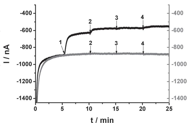
Fig. 18. Chronoamperometric response (in current density values) upon consecutive additions of L-lactate for two biosensors based on wild type (black line) and recombinant (grey line) *H. polymorpha* cells. Working electrode (graphite) polarized at -300 mV vs. Ag/AgCl 3M KCl. Additions 1-4, respectively: 1; 2.5; 5; 10 mM L-lactate.
