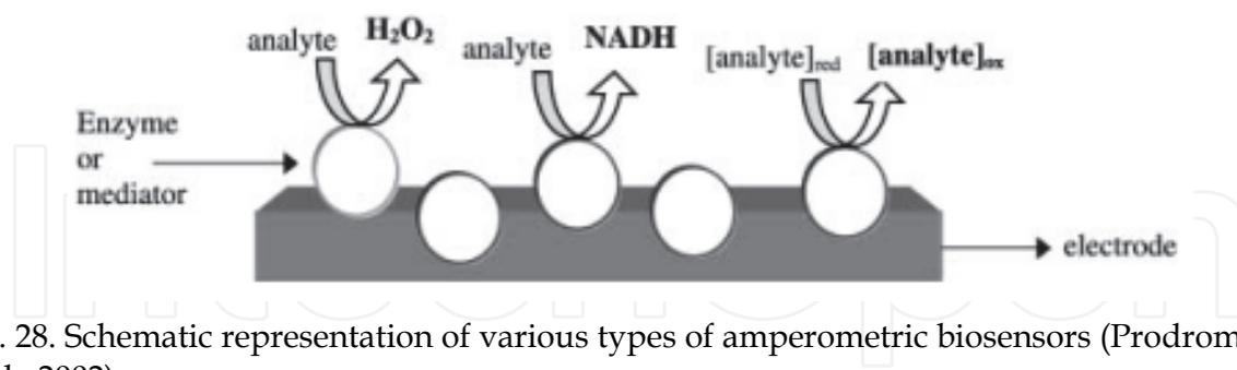
Fig. 28. Schematic representation of various types of amperometric biosensors (Prodromidis et al., 2002)
