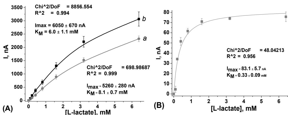
Fig. 13. (A) L-lactate calibration graphs for two types of sensors modified by genetically engineered *H. polymorpha* "tr1" cells (a - physical entrapment behind a dialysis membrane; b - electrochemically induced entrapment within a cathodic electrodeposition polymer CP9); (B) L-lactate calibration graph for sensor modified by *H. polymorpha* "C-105" cells by physical entrapment behind a dialysis membrane.
