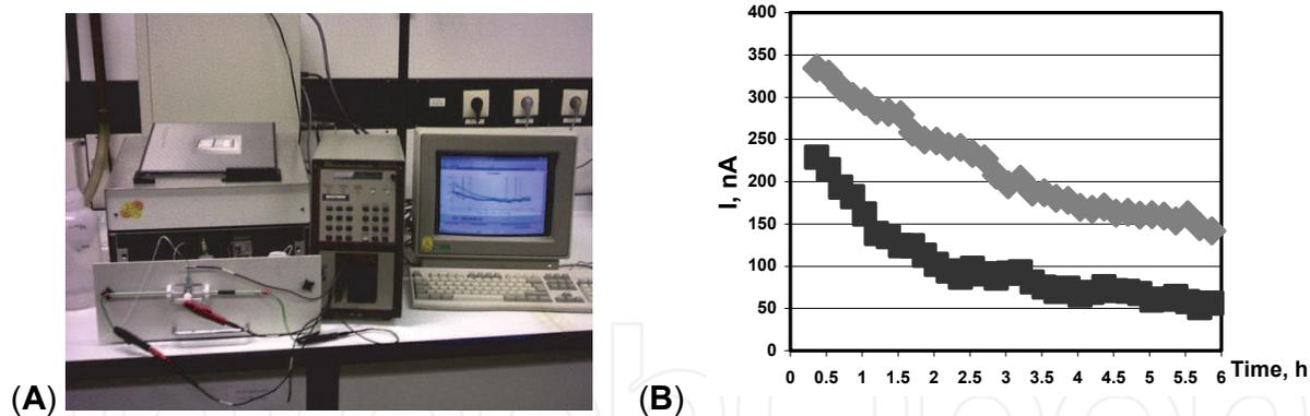
Fig. 9. Flow injection “OLGA” analyzer system with integrated bioelectrodes (A) and operation stability of the sensor obtained by “OLGA” (1 mM L-Lactate, flow-rate 5 ml min<sup>-1</sup>, 24 °C and detection of results every 4 min) (B).
