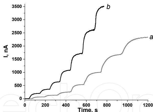
Fig. 12. Chronamperometric current response upon subsequent additions of L-lactate aliquots obtained with microbial sensors based on permeabilized cells of the recombinant strain of *H. polymorpha* ("tr1"). (a) Immobilization of cells by means of physical entrapment behind a dialysis membrane. (b) Entrapment of cells within a layer of a cathodic electrodeposition polymer CP9. (3.05 mm diameter graphite disk electrode; 0 mV vs. Ag/AgCl).
