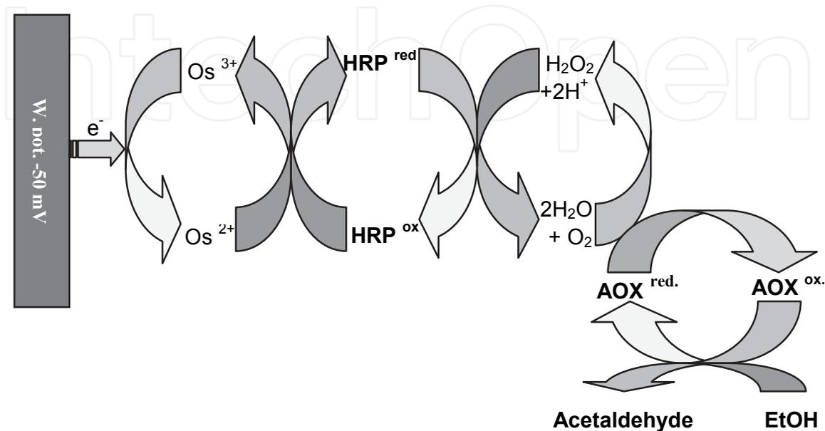
Fig. 19. Reaction scheme and electron-transfer pathway from ethanol *via* AOX, enzymatically generated H<sub>2</sub>O<sub>2</sub>, HRP, and polymer-bound Os-relays to the electrode.
