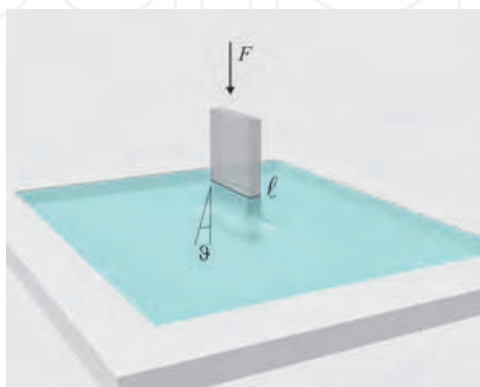
Fig. 4. Scheme and reference angle for Wilhelmy equation.
