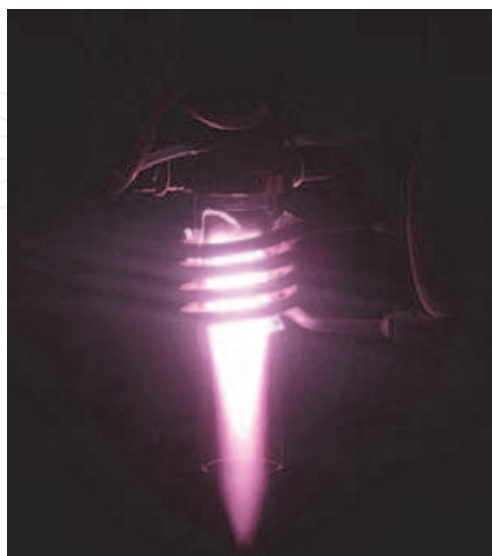
Fig. 1. Photograph of induction plasma generated by argon discharge
