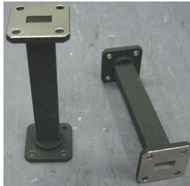
Fig. 4. Rectangular waveguides with width a = 1.30 cm and height b = 0.64 cm.
