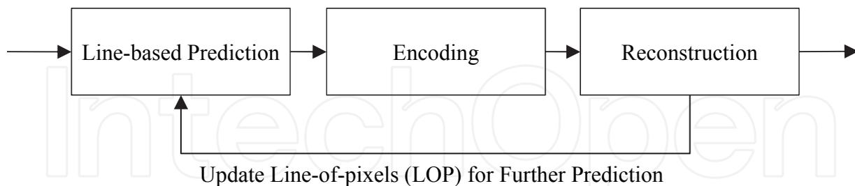
Fig. 6. Line-based prediction process.
