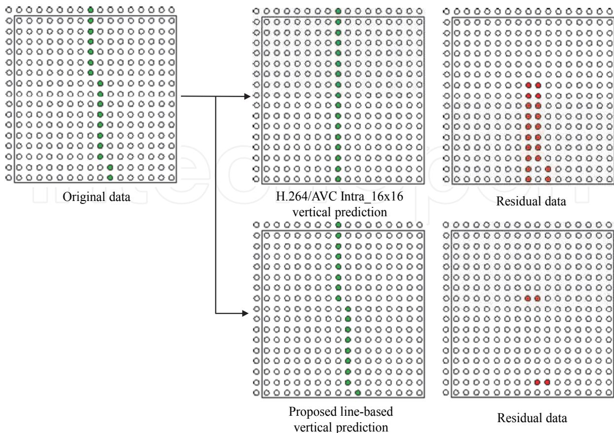
Fig. 11. Prediction result comparison between the conventional Intra<sub>16</sub>×16 and proposed line-based Intra<sub>16</sub>×16 predictions.
