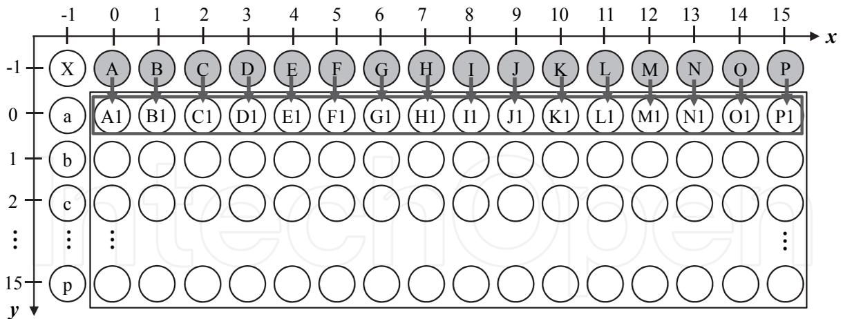
(a) Vertical mode of the Intra<sub>16</sub> × 16 mode
