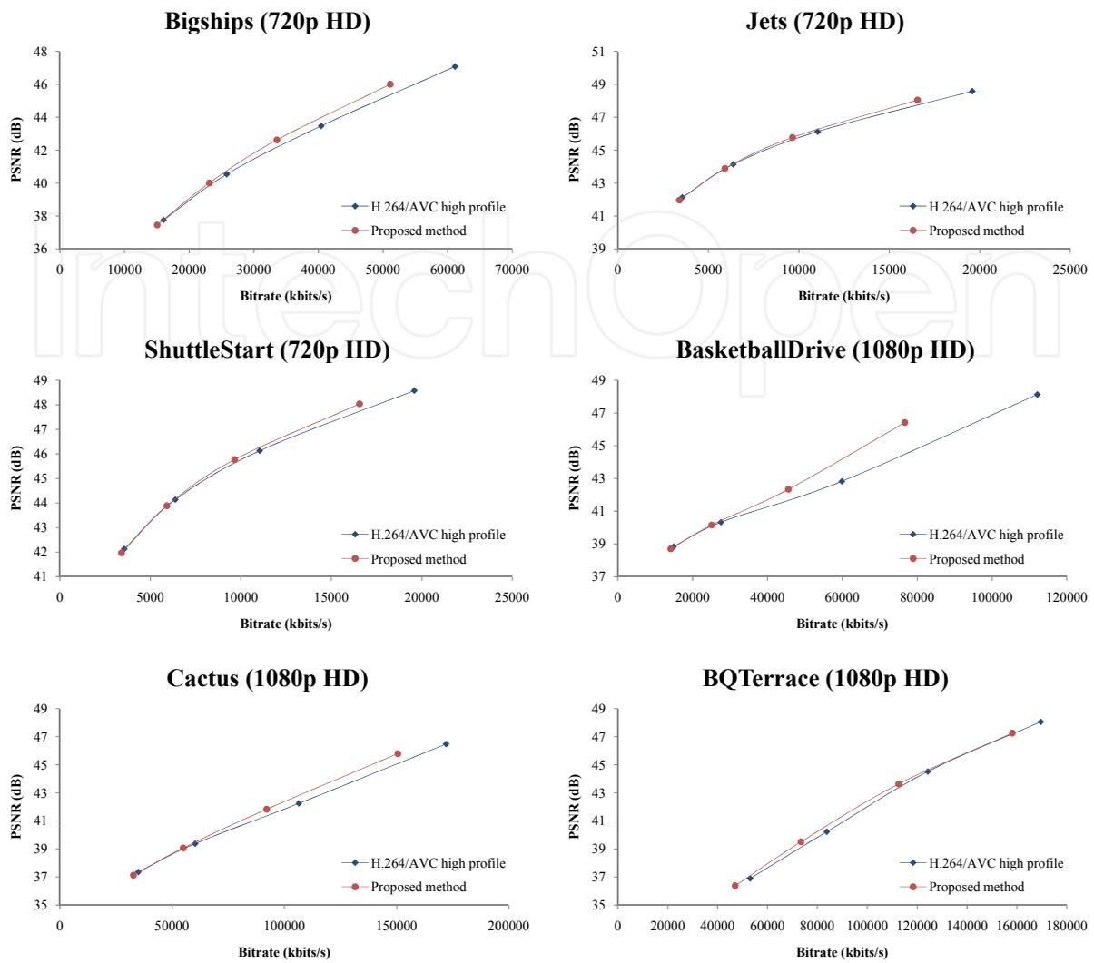
Fig. 12. Rate-distortion curve of proposed technique.
