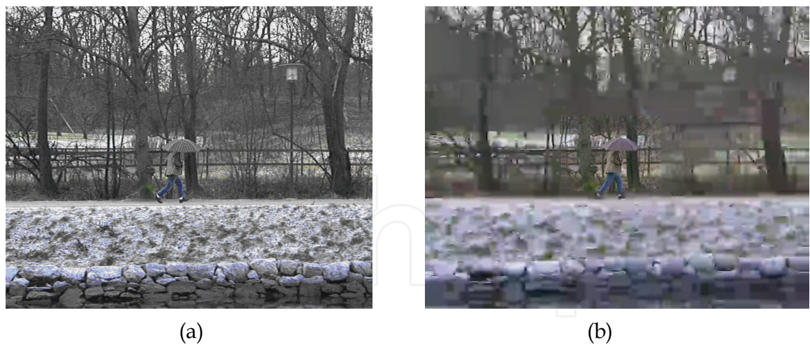
Fig. 12. The "PARKRUN" video sequence containing the ROI region in the middle of the frame – the man with an umbrella (the quantization parameter of the background region can be determined adaptively); (a) the original frame; and (b) the compressed frame with the higher-quality ROI region.
