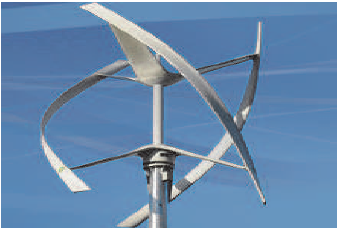
Fig. 3. VAWT made by Urban Green Energy
