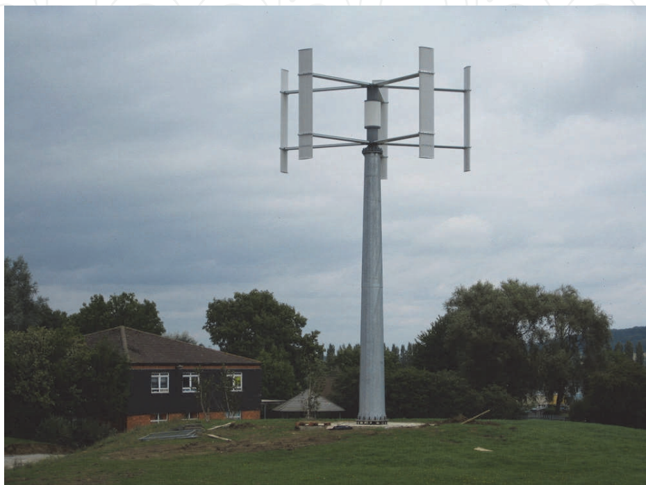
Fig. 4. H-type VAWT made by Ropatec of Italy
