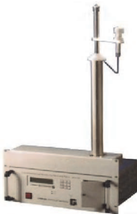
Fig. 7. Measuring equipment for taking particulate matter measurements Source: Grimm # 180 dust monitor manual
