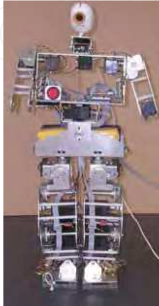
Figure 12. Biped humanoid robot with 22 DOFs
