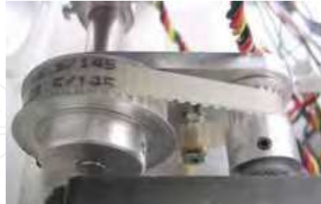
Figure 3. Transmission with a 2.5:1 gear ratio; an adjustable tensile roller holds the belt tight
