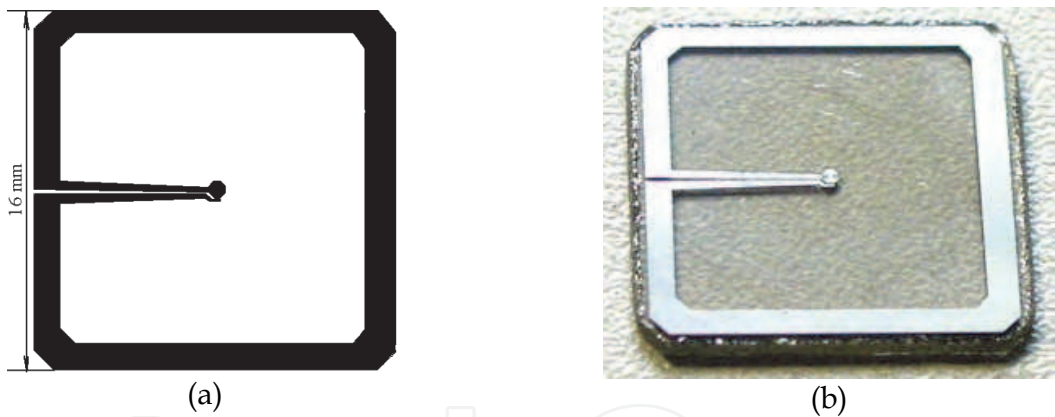
Fig. 11. (a) Sketch and (b) photograph of 16-mm high- T_c superconducting multilayer flux transformer with multiturn input coil in the middle intended for a 16-mm high- T_c DC SQUID flip-chip magnetometer.
