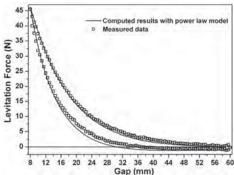
Fig. 6. Comparison of the levitation force versus gap curve between the computed results and measured results under vertical movement in the applied field generated by Rail\_1 shown in Fig. 4. The Y-Ba-Cu-O was bath-cooled at a position which was 60 mm above the rail where the applied field is weak and so this case can be approximately considered as zero field-cooled condition.
