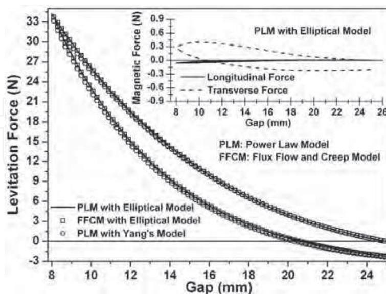
Fig. 5. Comparison of levitation force versus gap curve between different  $E$ - $J$  constitutive relations and angular-dependent of the critical current density formulations as well as the transverse and longitudinal force versus gap behavior with power law and elliptical model (inset). The applied field was provided by Rail\_1 shown in Fig. 4.
