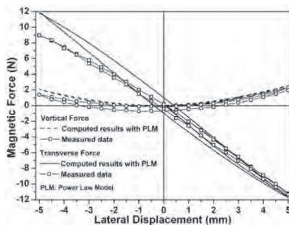
Fig. 10. Comparison of the magnetic force as a function of lateral displacement between the computed and measured results under transverse movement in the applied field generated by Rail\_2 shown in Fig. 4. The Y-Ba-Cu-O sample was field-cooled at the identical height (18 mm) with the levitation height where the magnetic force was calculated or measured.
