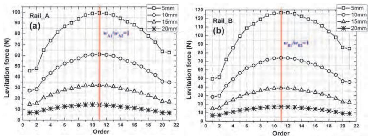
Fig. 14. The changing curve of the levitation force on the high-Tc superconductors at position of 5, 10, 15 and 20 mm above the Rail\_A (a) and Rail\_B (b) with the growth of the width ratio. The width ratio is replaced by an order and the corresponding relationship between the width ratio and the order (abscissa) is given in Table 5.
