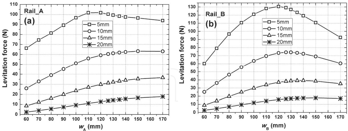
Fig. 16. The changing curve of the levitation force on the high-Tc superconductors at positions of 5, 10, 15 and 20 mm above the Rail\_A (a) and Rail\_B (b) with the growth of the total width. The total width was varied from 60 to 170 mm.
