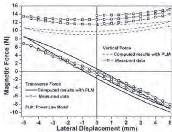
Fig. 9. Comparison of the magnetic force as a function of lateral displacement between the computed and measured results under transverse movement in the applied field generated by Rail\_2 shown in Fig. 4. The Y-Ba-Cu-O sample was field-cooled at a position of 30 mm, and the levitation gap where the magnetic force was calculated or measured was 18 mm above the rail.
