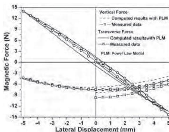
Fig. 11. Comparison of the magnetic force as a function of lateral displacement between the computed and measured results under transverse movement in the applied field generated by Rail\_2 shown in Fig. 4. The Y-Ba-Cu-O sample is field-cooled at a position of 13 mm, which was below the levitation gap (18 mm) where the magnetic force was calculated or measured.
