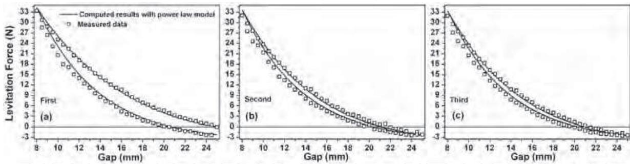
Fig. 7. Comparison of the levitation force versus gap curve between the computed results and measured results under vertical movement in the applied field generated by Rail\_1 shown in Fig. 4. The Y-Ba-Cu-O was bath-cooled at a position of 25 mm above the rail which was a typical field-cooled condition. The levitation force versus gap curve was calculated and measured with continuous three times here.
