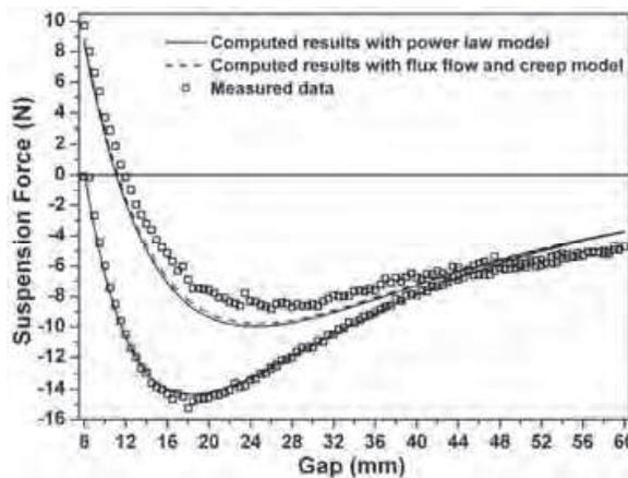
Fig. 8. Comparison of the suspension force versus gap curve between the computed results and measured results under vertical movement in the applied field generated by Rail\_1 shown in Fig. 4. The Y-Ba-Cu-O is bath-cooled at a position of 8 mm above the rail.
