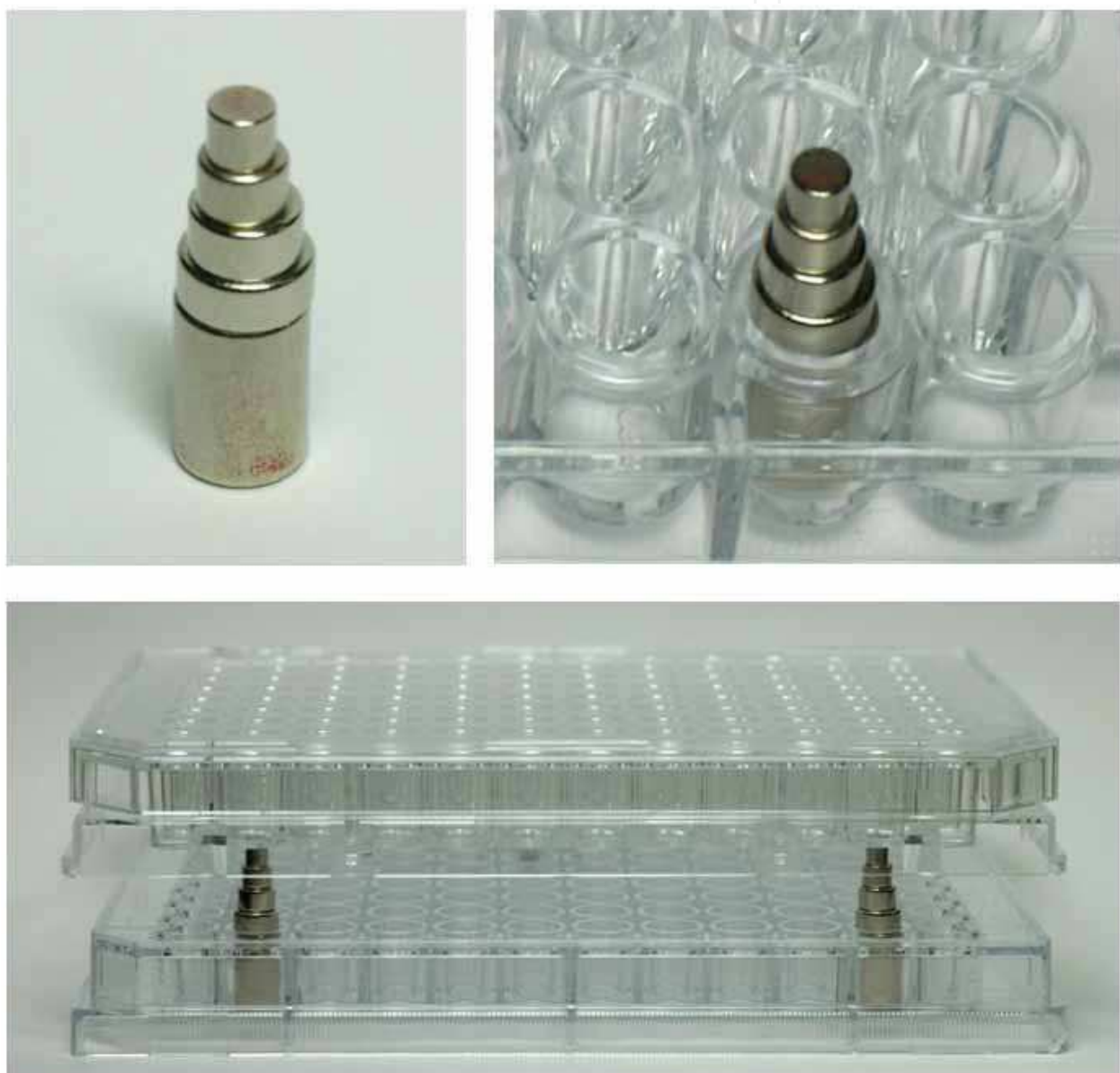
Fig. 11. The magnetic guidance of the magnetic nanoparticles using 96 well microplates.
