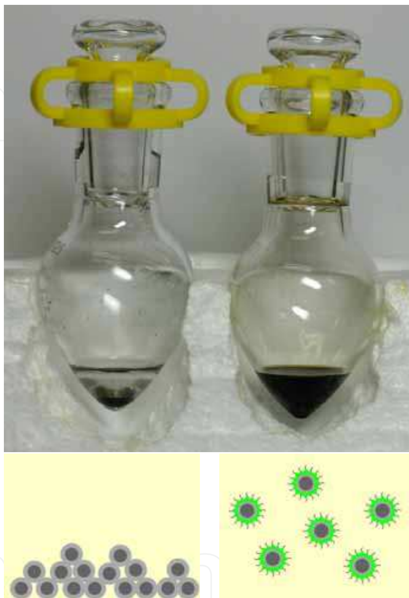
Fig. 5. Dispersion of the oleic acid-coated \text{Fe}_{16}\text{N}_2 / metallic oxide nanocomposite in chloroform. The magnetic fluid ( right ) was composed of the oleic acid ( green )-coated iron nitride/ metallic oxide nanocomposite ( dark gray/light gray ) dispersed in chloroform ( yellow ).
