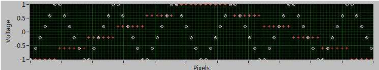
Fig. 4. Bi-direction scanning scheme. White (o): voltage applied onto X axis (fast) versus time (pixel sequence); red (+): voltage applied onto Y axis (slow) versus time (pixel sequence). The data collection of each pixel is synchronized with the scan control (Chen, Feng et al. 2010).
