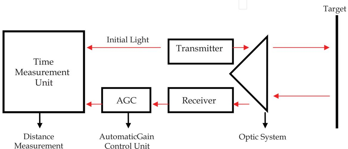
Fig. 2.5. Laser Telemetry Block Layout
