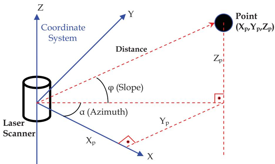
Fig. 2.6. TLS Local Coordinate System
