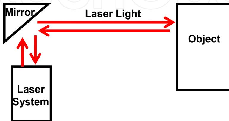
Fig. 2.3. Distance Measuring Method Based on Time of Flight
