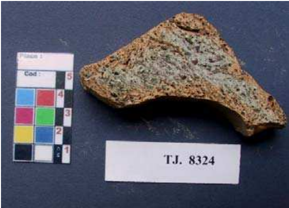
Fig. 1. Ceramic with different colors in the matrix as a function of uncontrolling firing.
