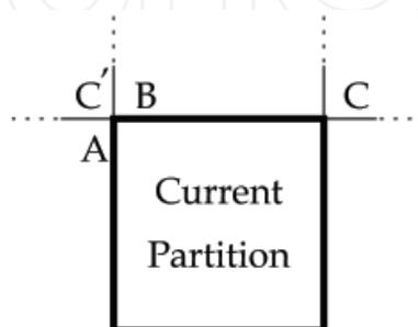
Fig. 3. Motion vectors of block  $A$ ,  $B$  and  $C$  are used for motion vector prediction. For DMVD predictive search,  $A$  and  $C$  ( $C'$  if  $C$  is unavailable) are used for motion derivation.
