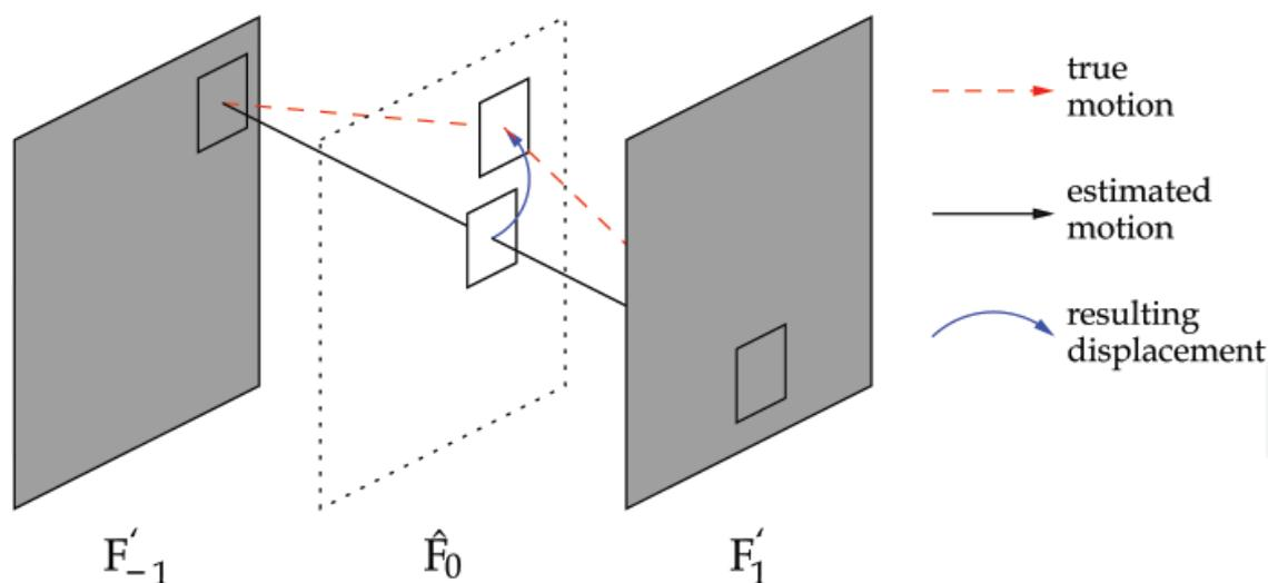
Fig. 7. Displaced interpolation due to nonlinear motion.
