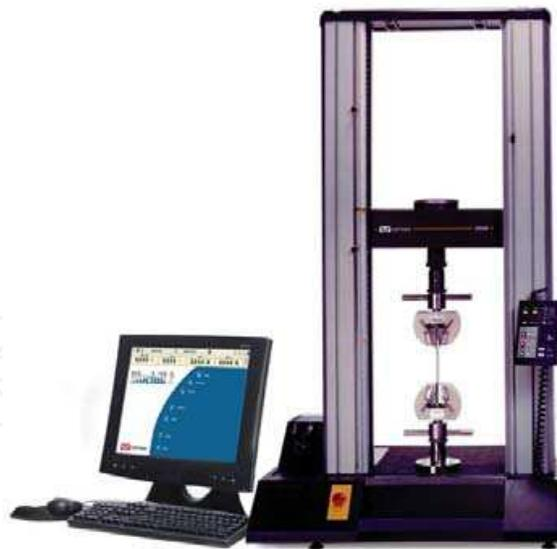
Fig. 12. Instron 5560 series instrument (<http://instron.itrademarket.com>)
