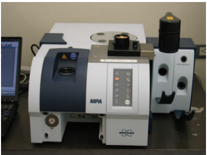
Photo 3. An instrument: The FT-NIR spectrometry MPA
