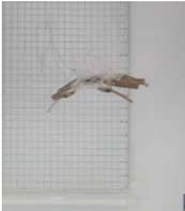
Fig. 20. Floating motion of the eight-legged microrobot
