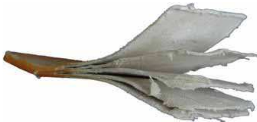
Fig. 15. Delaminated technical composite structure © PBGF.
