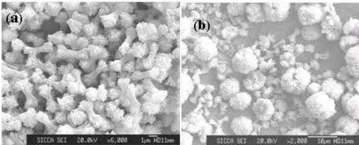
Fig. 12. SEM micrographs of  $\text{SrCO}_3$  prepared by microwave heating an aqueous solution of  $(\text{NH}_4)_2\text{CO}_3$  and  $\text{Sr}(\text{NO}_3)_2$  at  $90^\circ\text{C}$ . (a) for 30 s, and (b) for 1 min. Reproduced with permission from J. Nanosci. Nanotechn. **2007**, 7, 4552. Copyright **2007** ASP.
