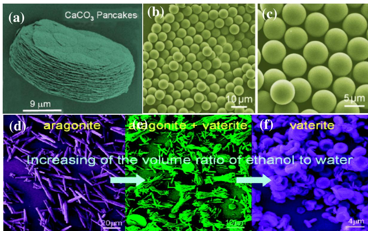
Fig. 29. SEM images of the  $\text{CaCO}_3$ : (a) calcite pancakes; (b,c) monodisperse  $\text{CaCO}_3$  (vaterite) microspheres; (d-f) vaterite superstructures and aragonite rods. Reproduced with permission from *Adv. Mater.* **2005**, *17*, 1461, *Angew. Chem. Int. Ed.* **2006**, *45*, 3977, and *Chem. Mater.* **2006**, *18*, 115. Copyright **2010** ACS and VCH.
