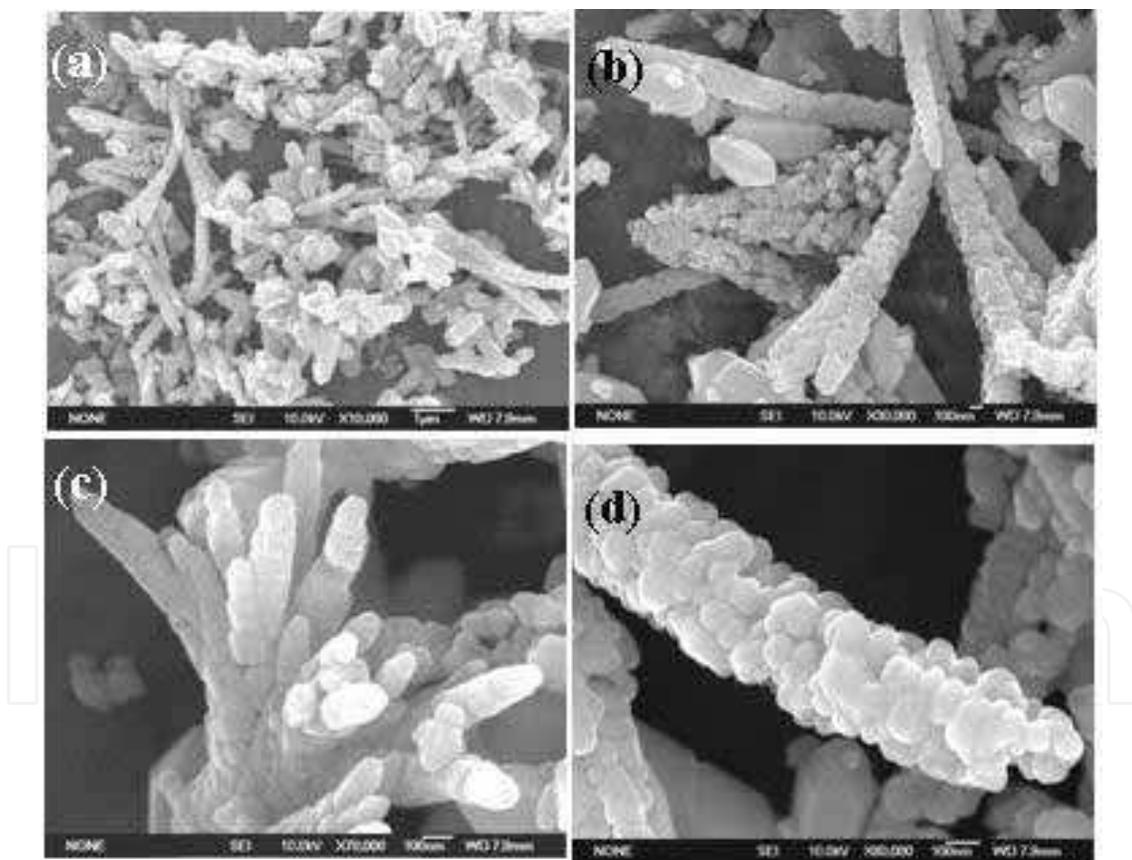
Fig. 13. SEM micrographs of  $\text{SrCO}_3$  prepared by microwave heating an aqueous solution of  $(\text{NH}_4)_2\text{CO}_3$ ,  $\text{Sr}(\text{NO}_3)_2$  and EDA at  $90^\circ\text{C}$  for 20 min. (a) at a lower magnification, (b) at a higher magnification, (c) the top view of the branch-like morphology, (d) a typical single branch assembled from nanoparticles. Reproduced with permission from Mater. Lett. **2008**, 62, 2512. Copyright **2008** Elsevier.
