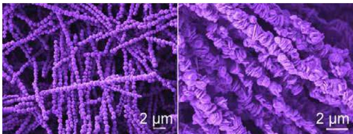
Fig. 28. SEM images of the one-dimensional assembly of  $\text{Ni}_x\text{Co}_{1-x}$  alloy microparticles. Reproduced with permission from Nano Research **2008**, *1*, 303. Copyright **2008** *springer*.
