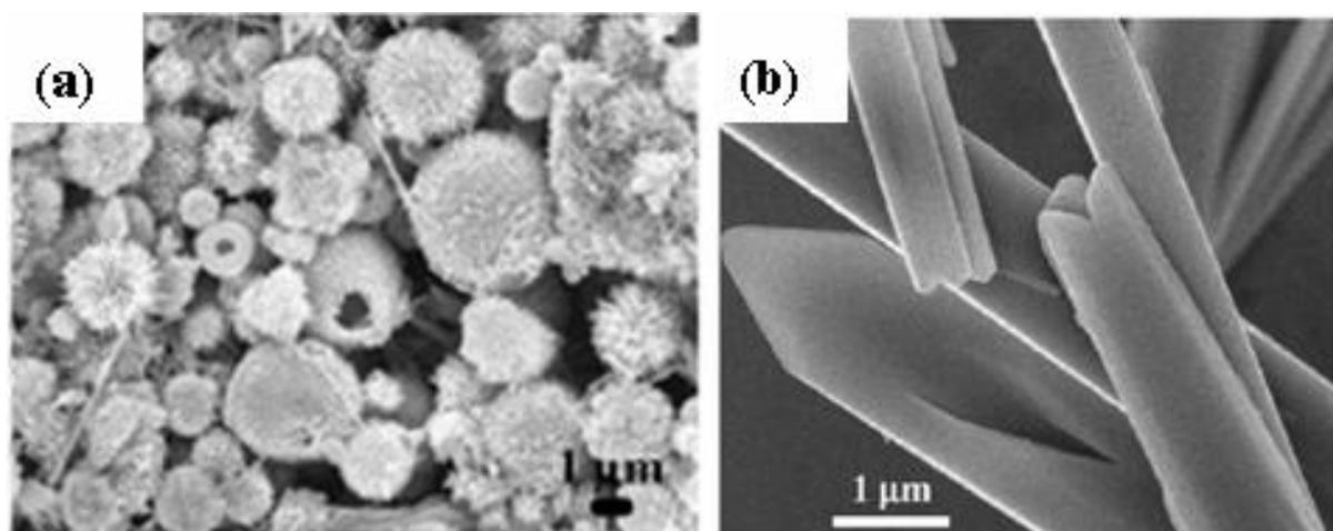
Fig. 1. (a) SEM micrograph of the hierarchically nanostructured HA hollow spheres, (Reproduced with permission from Eur. J. Inorg. Chem. **2009**, 5522. Copyright **2009** VCH.) and (b) TEM micrograph of the HA microtubes. (Reproduced with permission from Mater. Lett. **2008**, 62, 1642. Copyright **2008** Elsevier)
