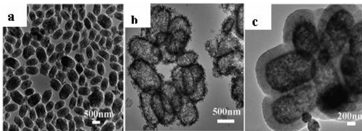
Fig. 3. TEM micrographs of (a)  $\text{CaCO}_3$  cores, (b) HA nanostructured hollow ellipsoidal capsules, (c) calcium silicate nanostructured hollow ellipsoidal capsules. Reproduced with permission from J. Mater. Chem., **2008**, *18*, 2722. Copyright **2008** RSC.
