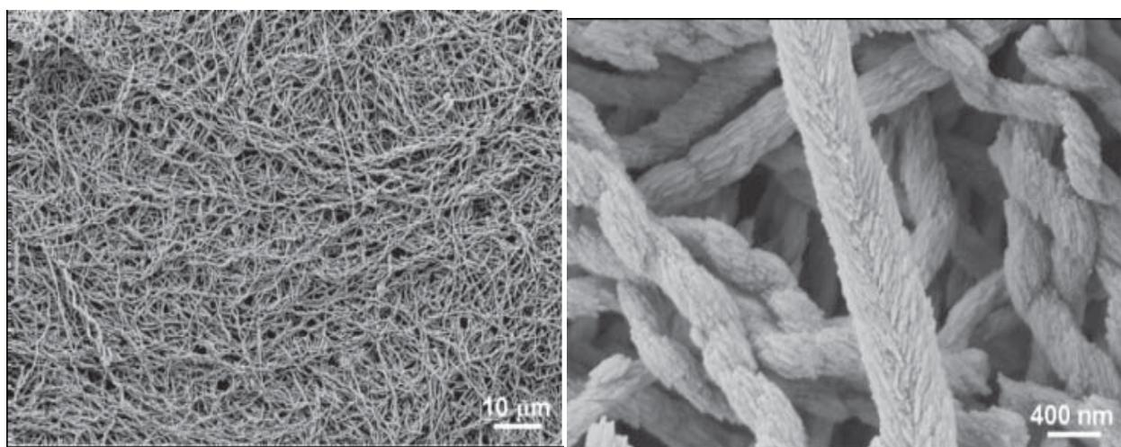
Fig. 25. Helical nanoparticle superstructures. **a**, The helical nanofibres formed at room temperature with PEG-b-DHPOBAEE,  $1 \text{ gL}^{-1}$ , starting  $\text{pH}=4$ ,  $[\text{BaCl}_2] = 10 \text{ mM}$ . **b**, Detailed surface structure. Reproduced with permission from *Nature Materials* **2005**, *5*, 51. Copyright **2005** Nature Publishing Group.
