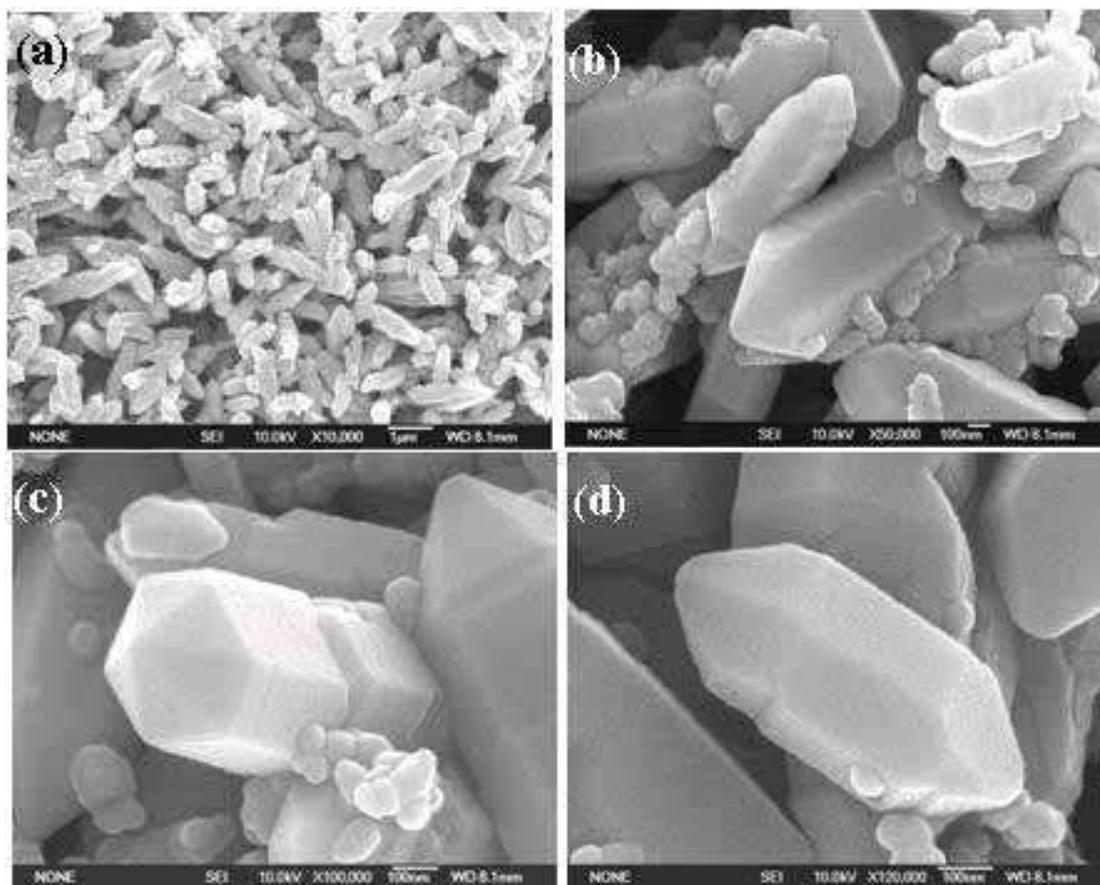
Fig. 14. SEM micrographs of  $\text{SrCO}_3$  prepared by microwave heating an aqueous solution of  $(\text{NH}_4)_2\text{CO}_3$ ,  $\text{Sr}(\text{NO}_3)_2$  and ethylenediamine at  $90^\circ\text{C}$  for 5 min. (a) at a lower magnification, (b) at a higher magnification, (c) the top view of the hexagonal cone, (d) a typical single hexagonal cone. Reproduced with permission from Mater. Lett. **2008**, *62*, 2512. Copyright **2008 Elsevier**.
