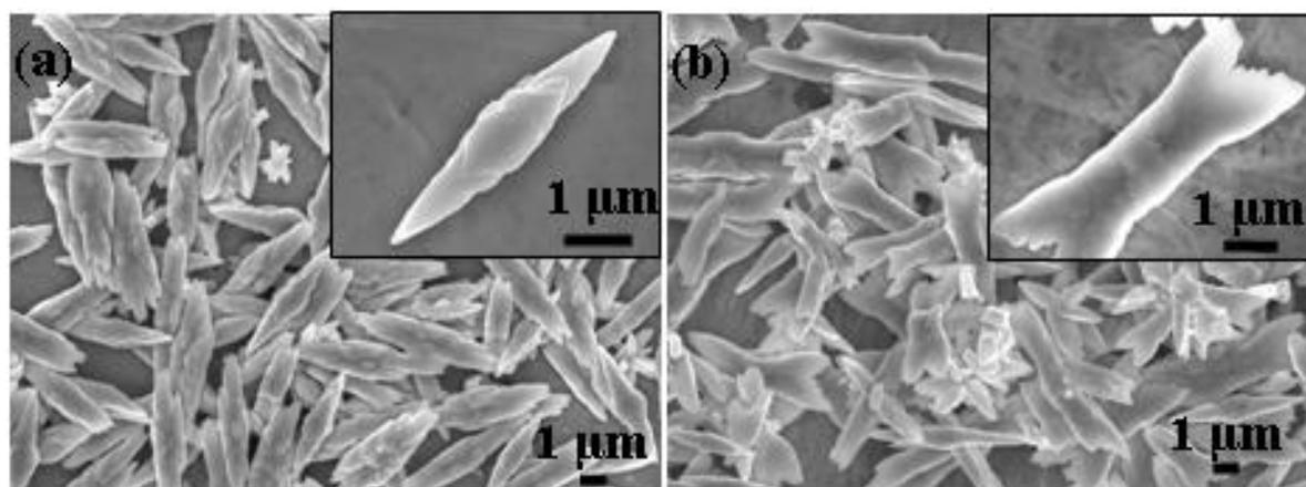
Fig. 17. SEM micrographs of  $\text{BaCrO}_4$  crystals prepared using different P123 concentration. (a)  $[\text{P123}] = 2.9 \text{ g L}^{-1}$  and (b)  $[\text{P123}] = 5.8 \text{ g L}^{-1}$ . The insets of (a) and (b) show the individual  $\text{BaCrO}_4$  crystals. Reproduced with permission from Mater. Res. Bull., **2009**, *44*, 288. Copyright **2009** Elsevier.
