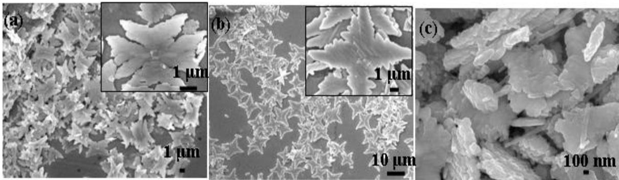
Fig. 18. SEM micrographs of  $\text{BaCrO}_4$  structures. (a) in the absence of P123; (b) in the absence of P123 and NaOH; (c) 15 mL  $0.58 \text{ g L}^{-1}$  P123,  $\text{Ba}(\text{NO}_3)_2$  concentration increased from 0.05 to  $0.20 \text{ mol L}^{-1}$  (0.5 mL), 1 mL  $0.50 \text{ mol L}^{-1}$  NaOH. Reproduced with permission from Mater. Res. Bull., **2009**, *44*, 288. Copyright **2009** Elsevier.
