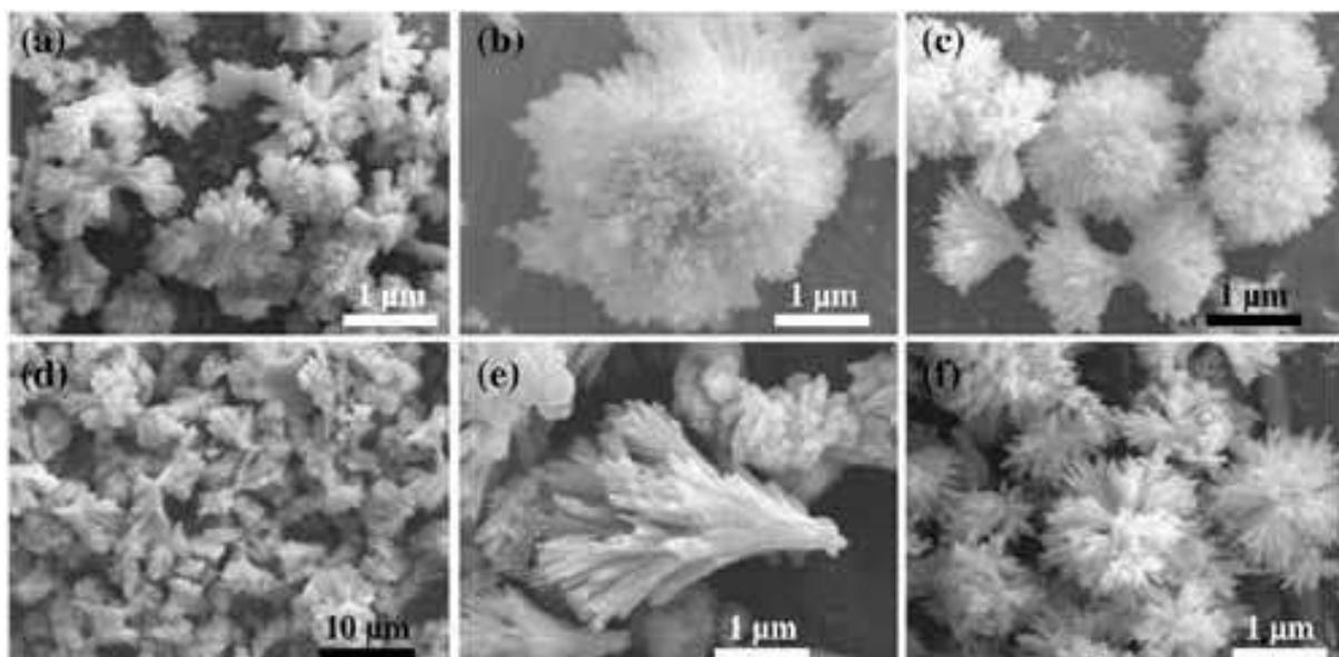
Fig. 9. SEM micrographs of the sample prepared using  $(\text{NH}_4)_2\text{CO}_3$  as the  $\text{CO}_3^{2-}$  source. (a) A typical SEM micrograph; (b) an individual flower-like structure. (c) using 20 mL 2.9 g/L P123; (d, e) using 20 mL SDBS (25.090 g/L); (f) using 20 mL CTAB (9.100 g/L). Reproduced with permission from Mater. Lett. 2008, 62, 3110. Copyright 2008 Elsevier.
