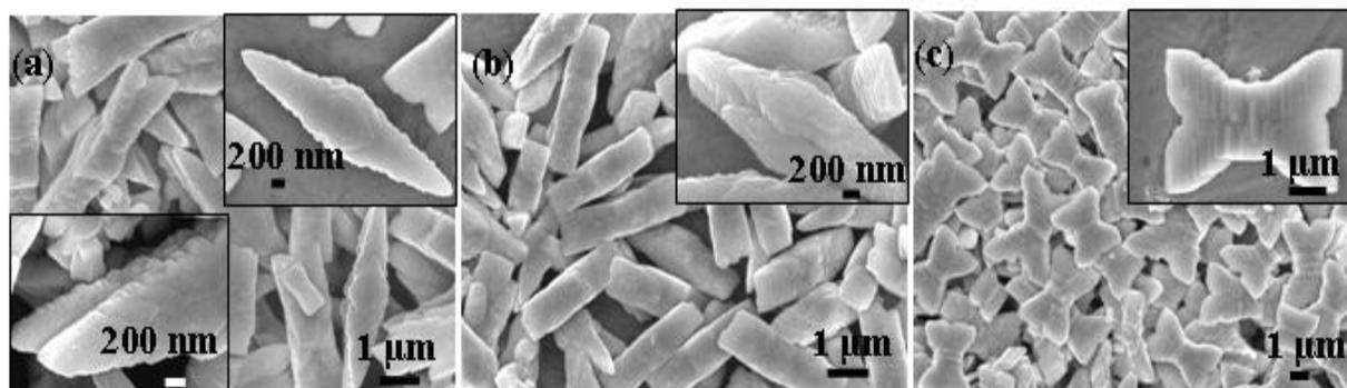
Fig. 16. SEM micrographs of  $\text{BaCrO}_4$  crystals prepared for different time. (a) 5 min; (b) 3 h; and (c) 6 h. Reproduced with permission from Mater. Res. Bull., **2009**, *44*, 288. Copyright **2009** Elsevier.
