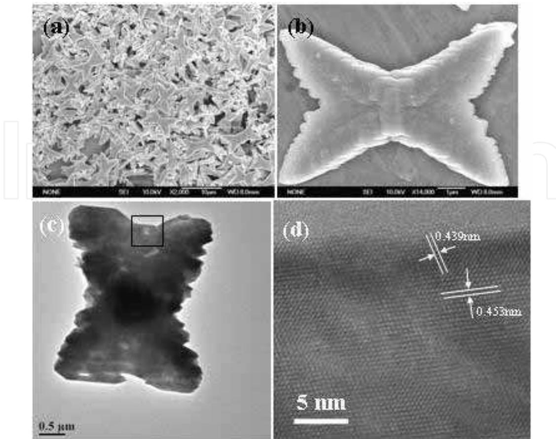
Fig. 15. (a) XRD pattern; (b) and (c) SEM micrographs; and (d) TEM micrograph of the typical  $\text{BaCrO}_4$  sample. The HRTEM image of the individual X-shaped structure shown in (d) is given in (e). Reproduced with permission from Mater. Res. Bull., **2009**, *44*, 288. Copyright **2009 Elsevier**.
