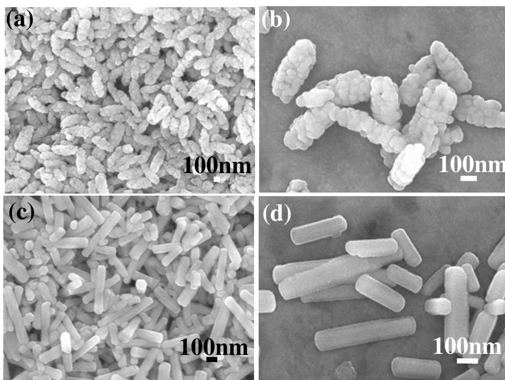
Fig. 6. SEM micrographs of  $\text{BaCO}_3$  prepared by microwave heating at  $90^\circ\text{C}$  for 40 min in ethylene glycol. (a,b) using NaOH, (c,d) using hexamethylenetetramine. Reproduced with permission from Chem. Lett. **2006**, *35*, 1138. Copyright **2006 CSJ**
