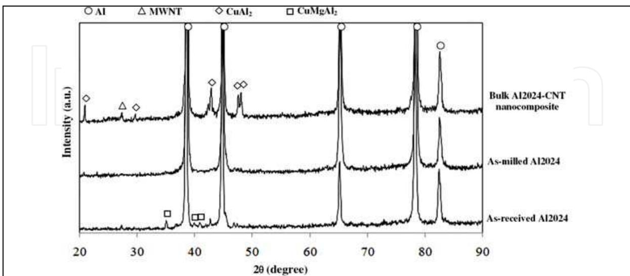
Fig. 4. XRD patterns of as-received Al2024 powders, 30h-milled Al2024 powders and bulk Al2024-3vol%MWCNTs nanocomposite
