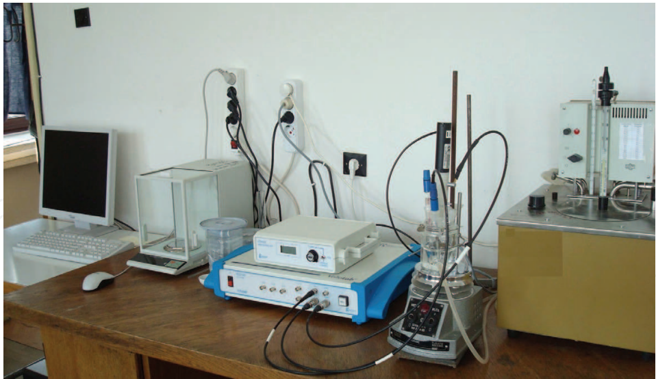
Fig. 1. Equipment Voltalab 10 for electrodepositions and some corrosion measurements
