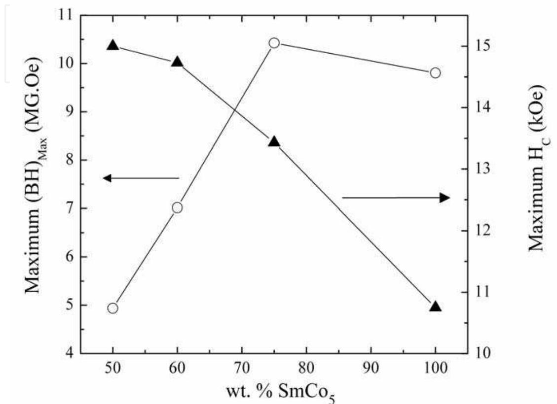
Fig. 8. Dependence of the maximum achievable values of coercivity,  $H_C$ , and energy product,  $(BH)_{\text{Max}}$ , as a function of the  $\text{SmCo}_5$  weight percentage. The values plotted correspond to the milling times that give maximum  $H_C$  and  $(BH)_{\text{Max}}$  for each composition.
