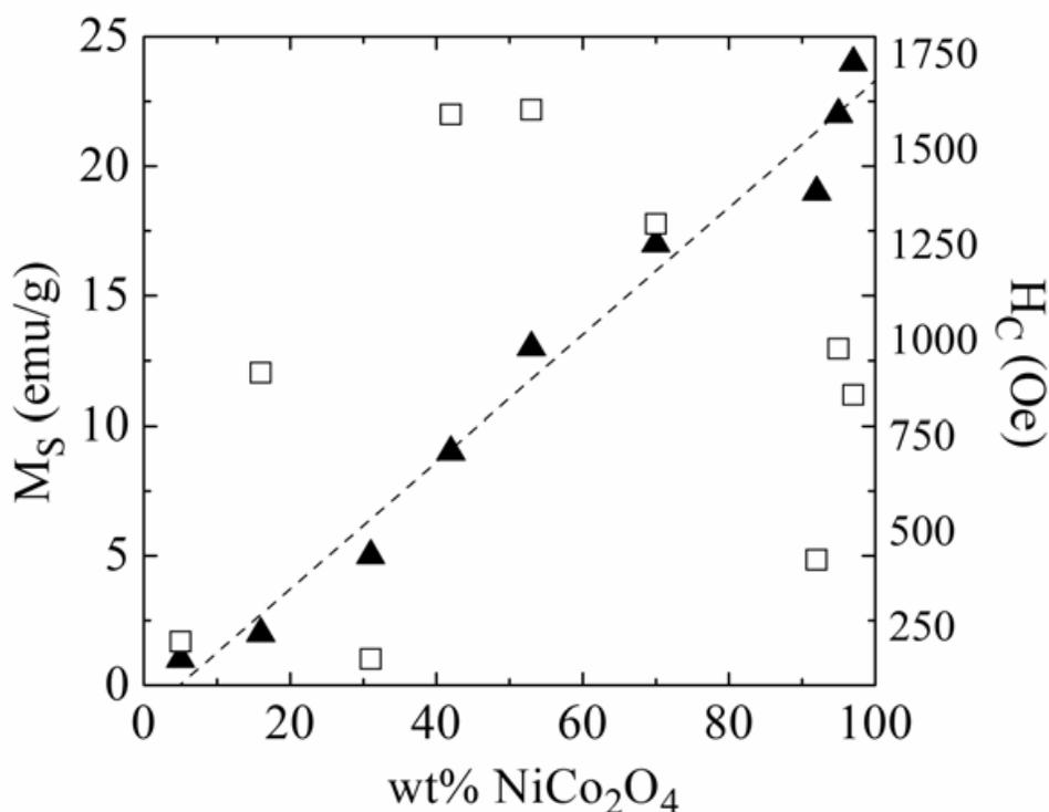
Fig. 11. Saturation magnetization (▲) and coercivity (□) (at  $T = 10$  K) dependence of the nanocomposites with the amount of FiM  $\text{NiCo}_2\text{O}_4$ . The amount of  $\text{NiCo}_2\text{O}_4$  was estimated by Rietveld refinement of the corresponding X-ray diffraction patterns. The dashed line is an eye-guide.
