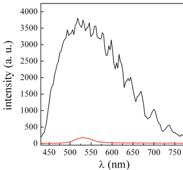
Fig. 15. Non-normalized PL spectra of SBA-16 SiO<sub>2</sub>@CdS composite (black curve) and *free* CdS nanocrystals (red curve). Notice the huge difference in intensity between both curves, especially taking into account that the SB6-16 SiO<sub>2</sub> host alone does not emit.
