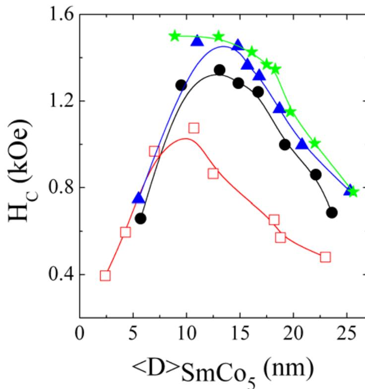
Fig. 5. Dependence of the coercivity,  $H_C$ , on the  $\text{SmCo}_5$  crystallite size (which is, in turn, tuned by varying the milling time) for  $\text{SmCo}_5$ :NiO milled in a weight ratio of 1:0 (-□-), 3:1 (-●-), 3:2 (-▲-) and 1:1 (-★-). The lines are a guide to the eye.
