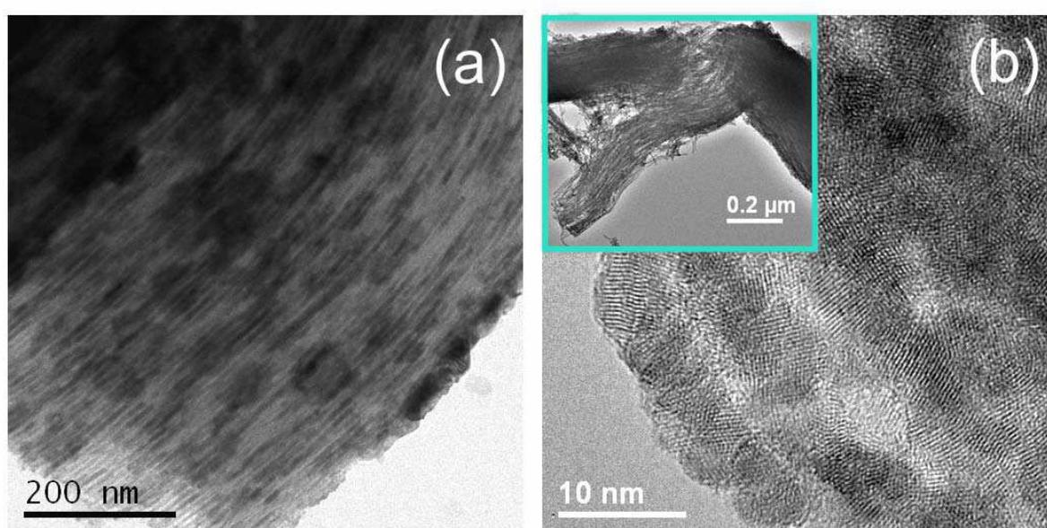
Fig. 13. TEM image of (a) SBA-15 SiO<sub>2</sub>@CdS composite and (b) *free* CdS nanocrystals in SBA-15 structure (a view at lower magnification is shown in the inset).
