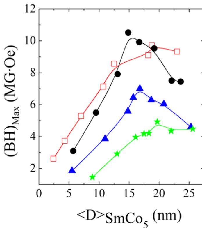
Fig. 7. Dependence of the energy product,  $(BH)_{\text{Max}}$ , on the  $\text{SmCo}_5$  crystallite size (which is, in turn, tuned by varying the milling time) for  $\text{SmCo}_5$ :NiO milled in a weight ratio of 1:0 (—□—), 3:1 (—●—), 3:2 (—▲—) and 1:1 (—★—). The lines are a guide to the eye.
