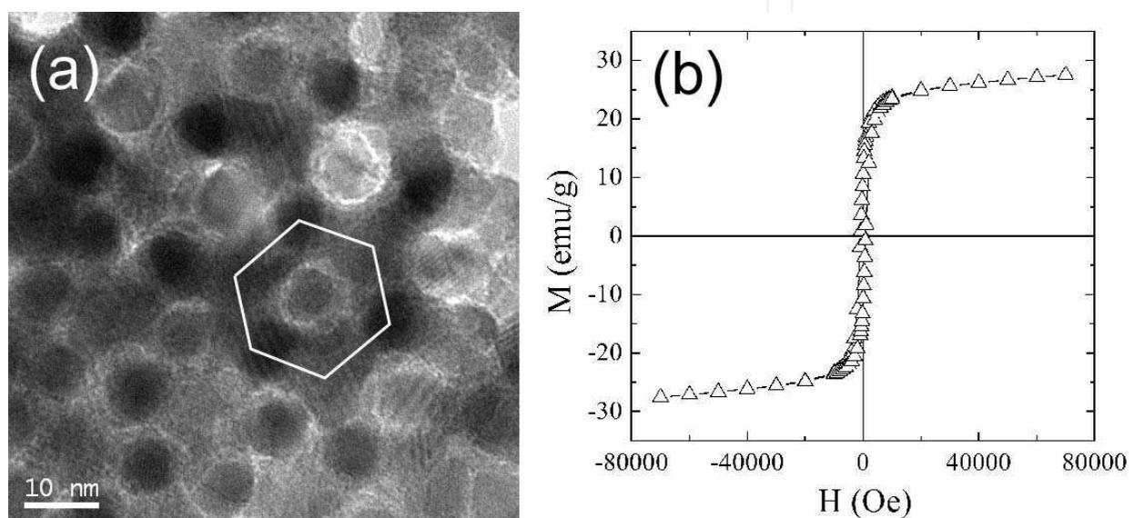
Fig. 12. (a) TEM image of a KIT-6 templated NiCo<sub>2</sub>O<sub>4</sub>-NiO (7 wt% NiO) composite (notice the hexagonal rings typical of this mesostructure) and (b) its corresponding hysteresis loop at 10 K.
