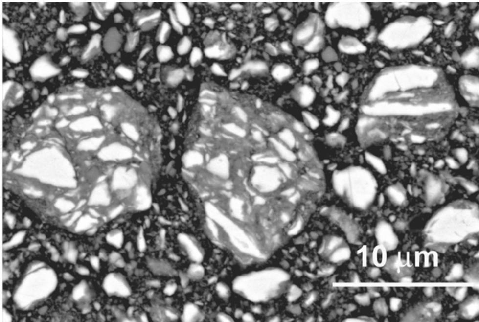
Fig. 3. Scanning electron microscopy image of SmCo<sub>5</sub> particles (light) embedded in a NiO matrix (grey). The image corresponds to SmCo<sub>5</sub> milled with NiO, for 32 h, in a weight ratio 1:1.
