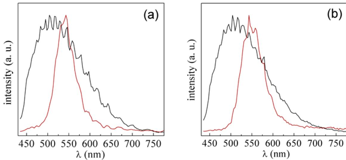
Fig. 14. Normalized PL spectra of (a) SBA-15 SiO<sub>2</sub>@CdS composite (black curve) and *free* CdS nanocrystals (red curve), (b) KIT-6 SiO<sub>2</sub>@CdS composite (black curve) and *free* CdS nanocrystals (red curve).
