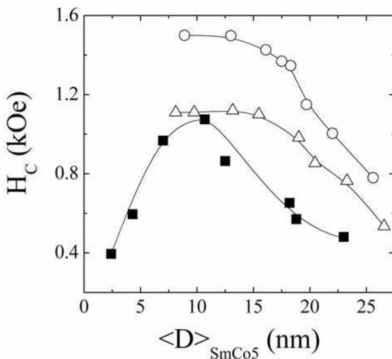
Fig. 6. Dependence of the coercivity,  $H_C$ , on  $\text{SmCo}_5$  crystallite size,  $\langle D \rangle_{\text{SmCo}_5}$ , for  $\text{SmCo}_5$  milled alone (—■—), with CoO (—△—) and NiO (—○—) in the weight ratio 1:1. The lines are a guide to the eye.
